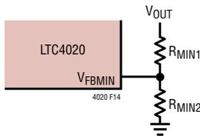
**Figure 14.  $V_{OUT}$  Instant-On Programming**
