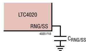
Figure 18. Using the RNG/SS Pin for Soft-Start
