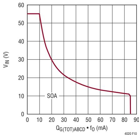
Figure 10.  $INTV_{CC}$  Pass Element SOA (Safe Operating Area)
