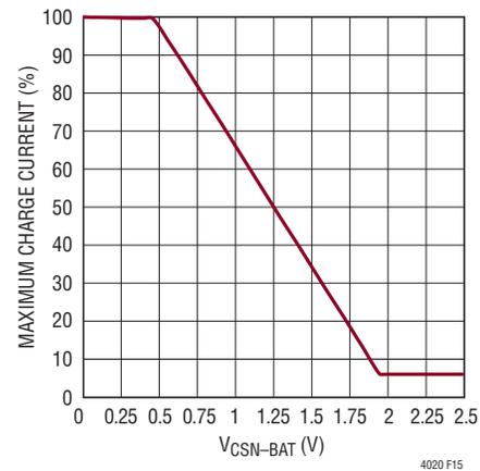
**Figure 15. Instant-On Charger Current Sense Limit Reduction**
