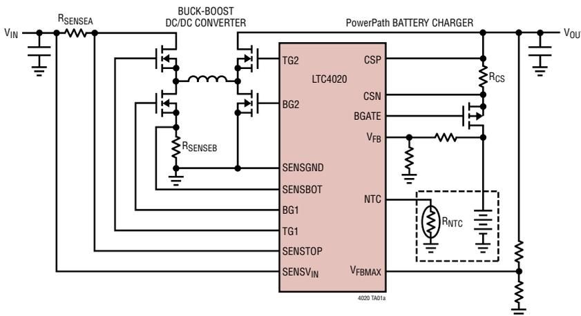
**5V to 30V 6-Cell Lead-Acid Supply/Charger
