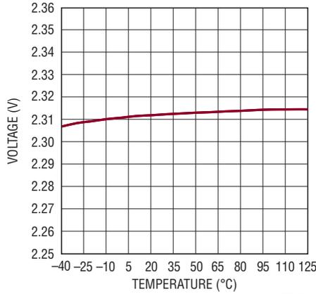
**$V_{\text{FBMAX}}$  Reference vs Temperature**
