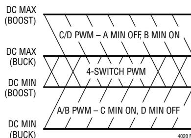
Figure 4. Operating Regions vs Duty Cycle (DC)
