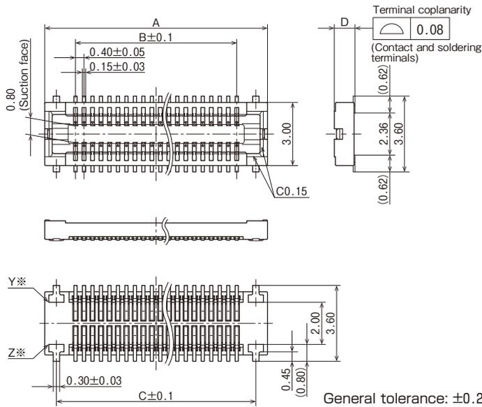
※Because the soldering terminal Y and Z are the unified structure, they are connected electrically.
