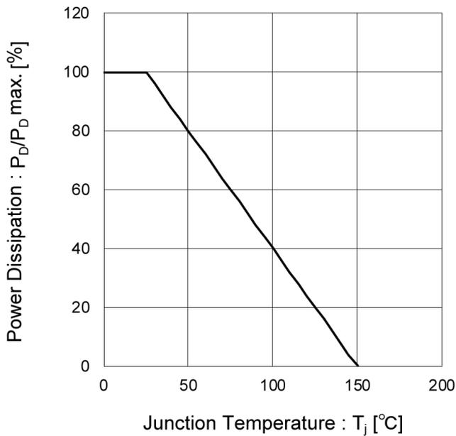
Fig.2 Drain Current Derating Curve vs. Junction Temperature
