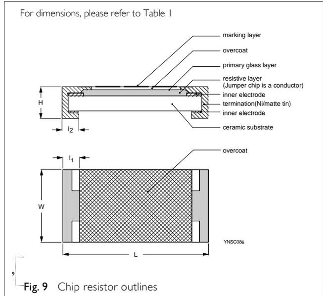
Fig. 9 Chip resistor outlines
