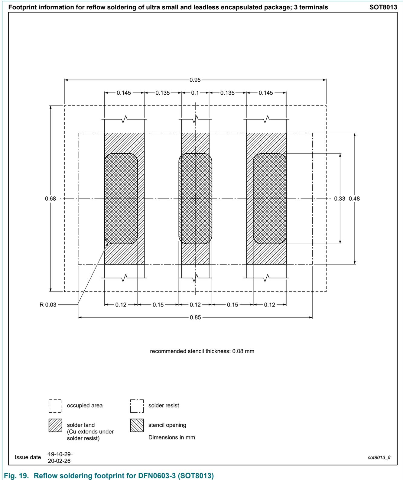
Fig. 19. Reflow soldering footprint for DFN0603-3 (SOT8013)
