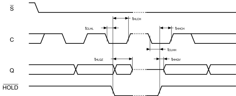
Figure 22. Serial output timing
