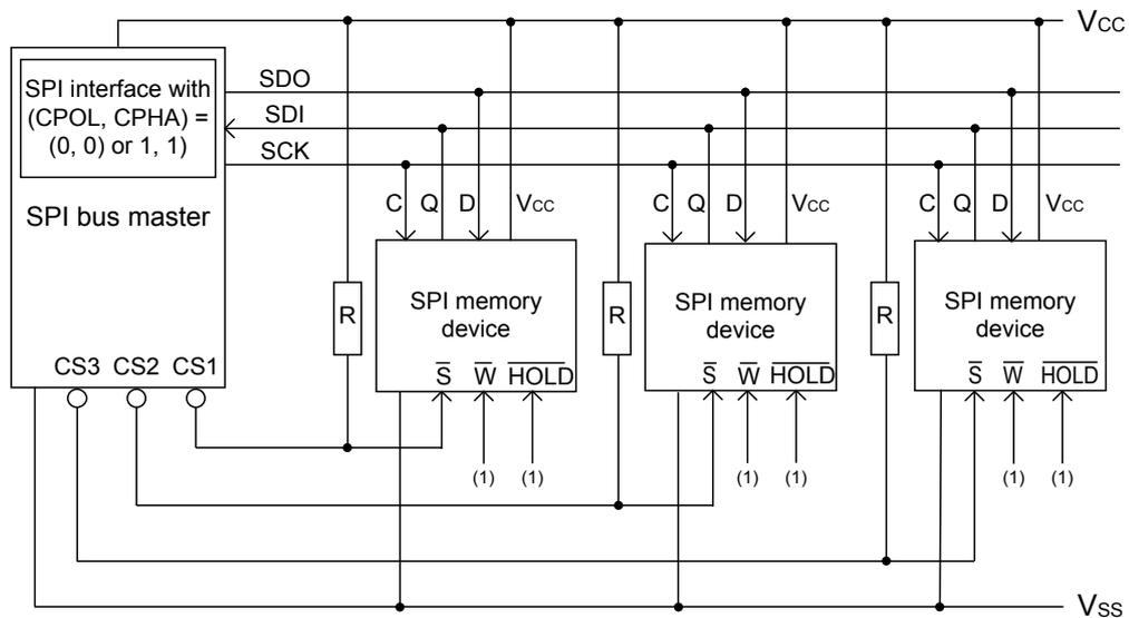
1. The Write protect ( $\bar{W}$ ) and Hold ( $\overline{HOLD}$ ) signals should be driven, high or low as appropriate.
