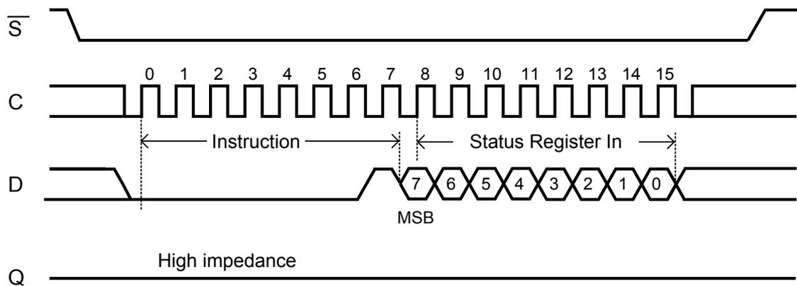
Driving the Chip select ( $\bar{S}$ ) signal high at a byte boundary of the input data triggers the self-timed Write cycle that takes  $t_W$  to complete (as specified in AC tables in [Section 9 DC and AC parameters](#)).
