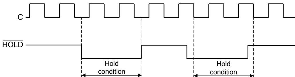
The Hold condition starts when the Hold ( $\overline{HOLD}$ ) signal is driven low when Serial clock (C) is already low (as shown in Figure 7).
