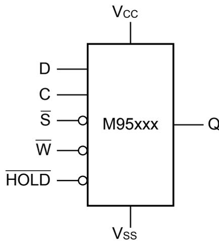
The SPI bus signals are C, D and Q, as shown in Figure 1 and Table 1. The device is selected when Chip select ( $\bar{S}$ ) is driven low. Communications with the device can be interrupted when the  $\overline{\text{HOLD}}$  is driven low.
