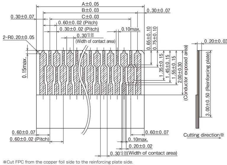
\*Cut FPC from the copper foil side to the reinforcing plate side.
