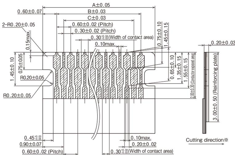
※Cut FPC from the copper foil side to the reinforcing plate side.
