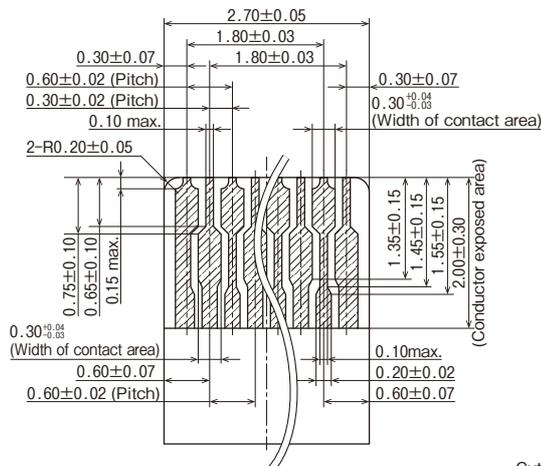
\*Cut FPC from the copper foil side to the reinforcing plate side.
