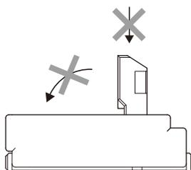
9) To close the lever, turn down the lever by pressing the entire lever or both sides of the lever with fingers tips. And close the lever completely. Be careful not to apply partial load to the lever that may cause its deformation or destruction or lever going back to initial position. Close the lever completely to prevent contact failure.
