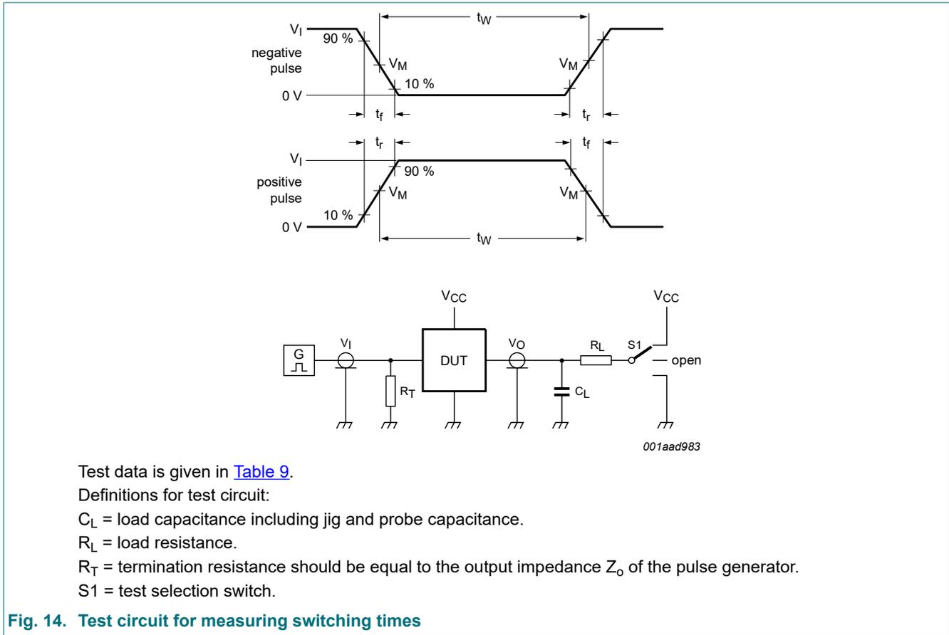
Fig. 14. Test circuit for measuring switching times
