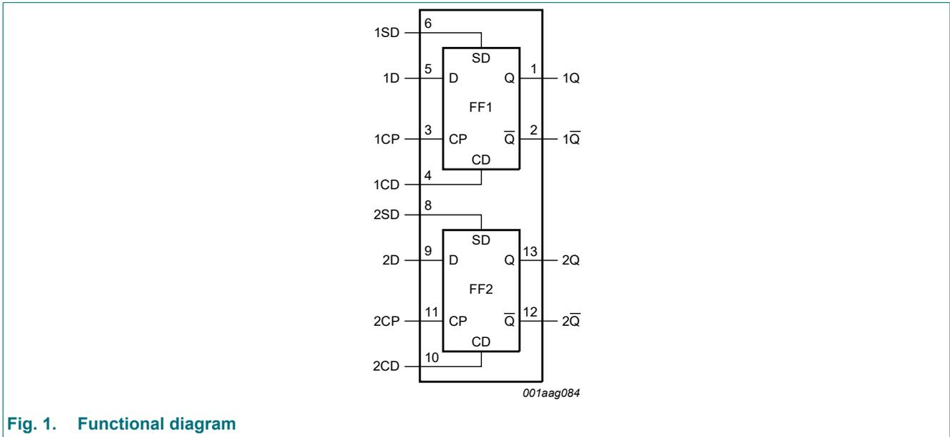
Fig. 1. Functional diagram
