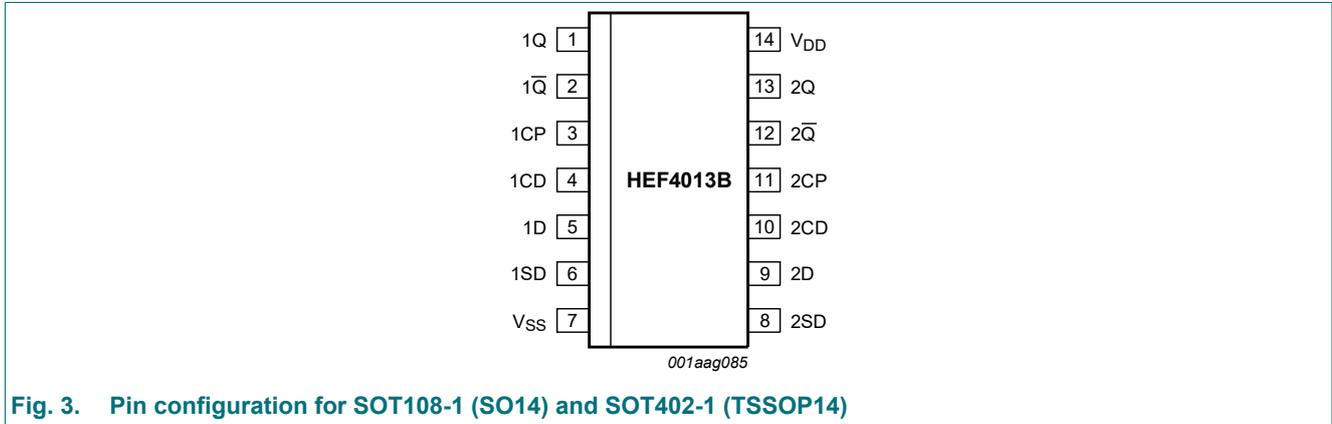
Fig. 3. Pin configuration for SOT108-1 (SO14) and SOT402-1 (TSSOP14)
