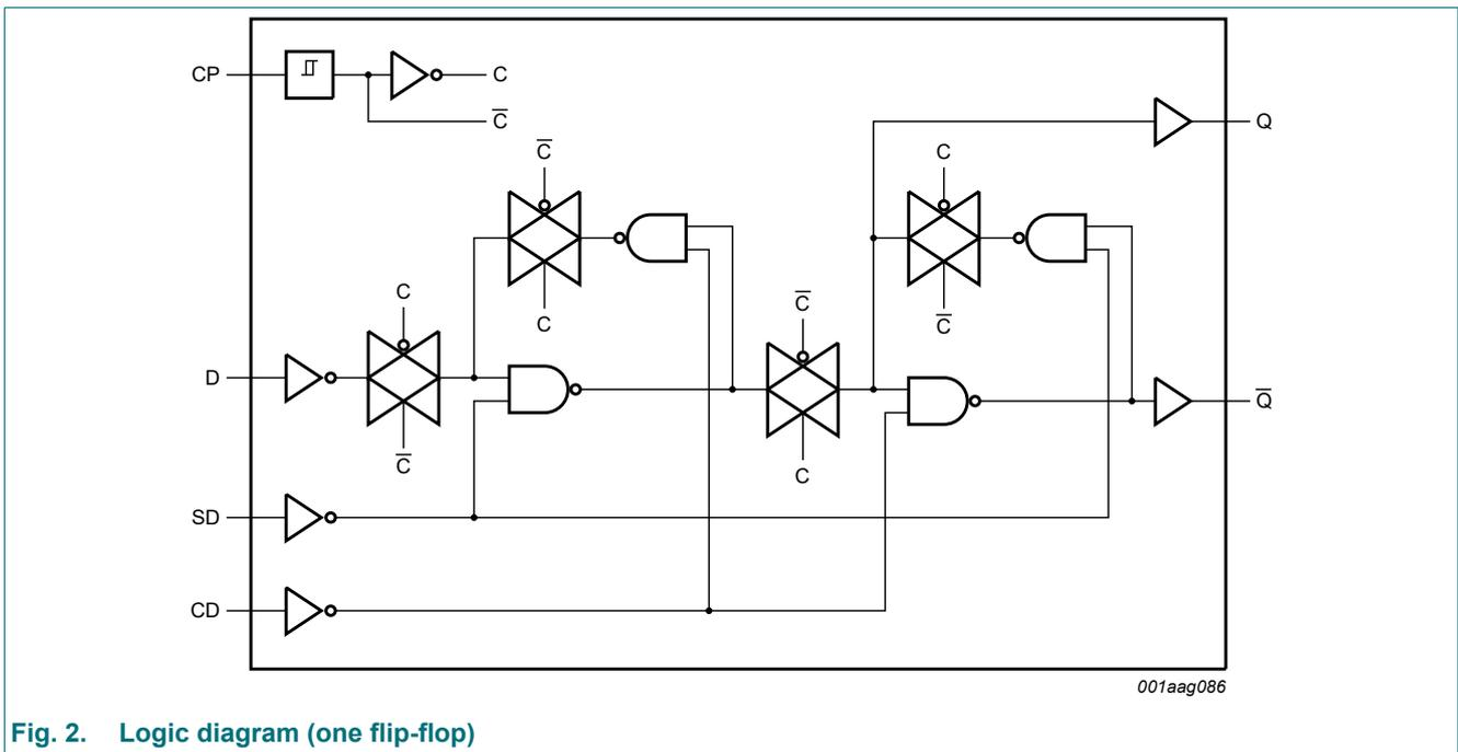
Fig. 2. Logic diagram (one flip-flop)
