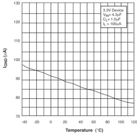
Fig. 9 Ground Current vs Temperature with 100µA Load
