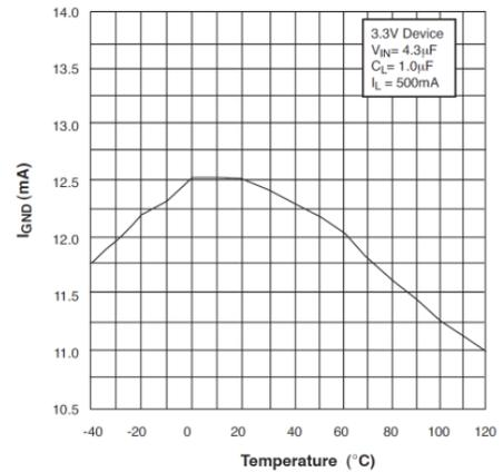
Fig. 12 Ground Current vs Temperature in Dropout
