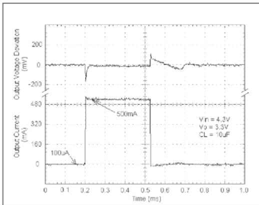
Fig. 17 Load Transient Response for 3.3V Device
