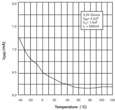
Fig. 11 Ground Current vs Temperature with 500mA Load
