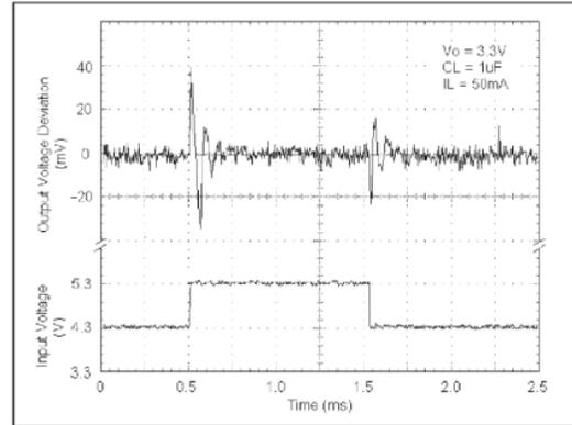
Fig. 16 Line Transient Response for 3.3V Device
