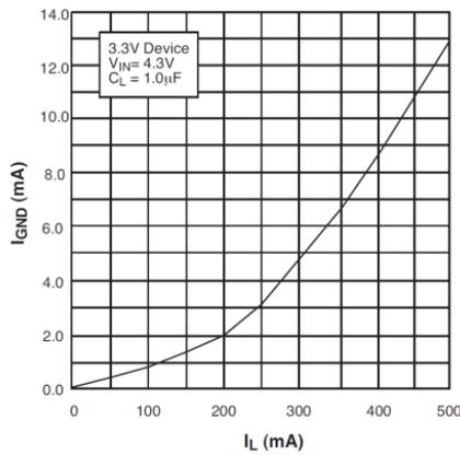
Fig. 5 Ground Current vs Load Current in Dropout
