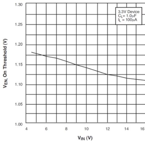
Fig. 13 ENABLE Voltage, ON threshold, vs Input Voltage
