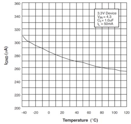
Fig. 10 Ground Current vs Temperature with 50mA Load
