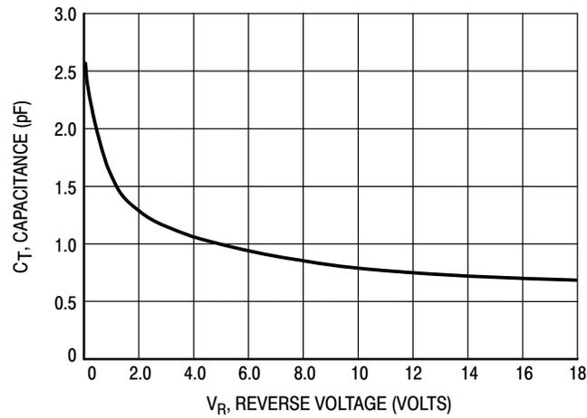
Figure 4. Typical Capacitance
