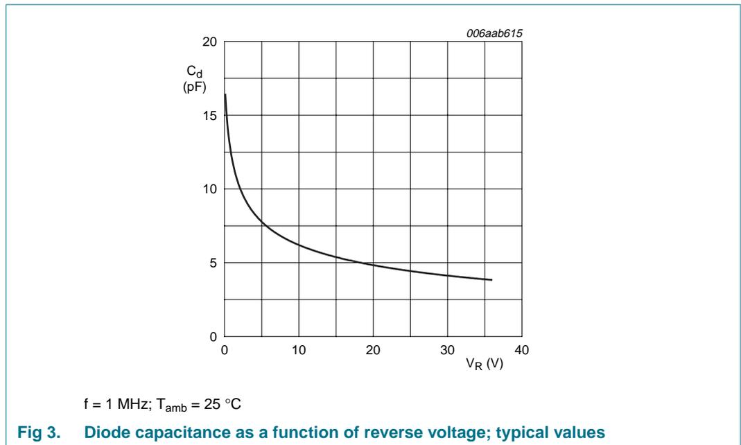
**Fig 3. Diode capacitance as a function of reverse voltage; typical values**
