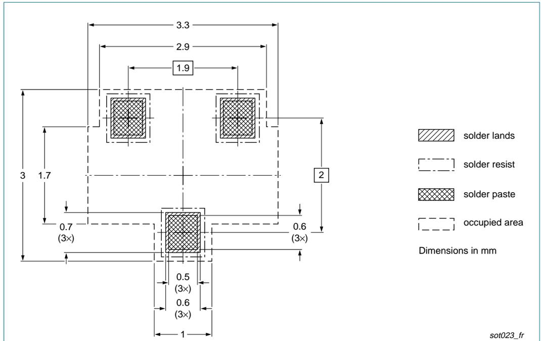
Fig 9. Reflow soldering footprint PESD36VS2UT (SOT23/TO-236AB)
