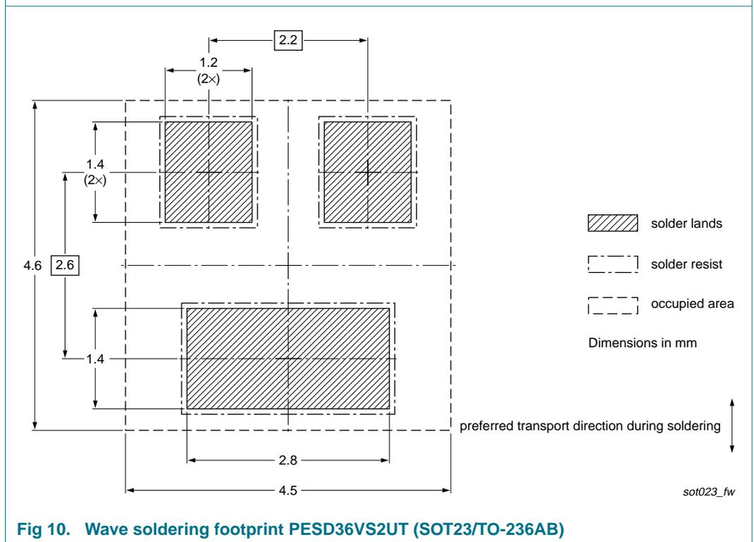
Fig 10. Wave soldering footprint PESD36VS2UT (SOT23/TO-236AB)
