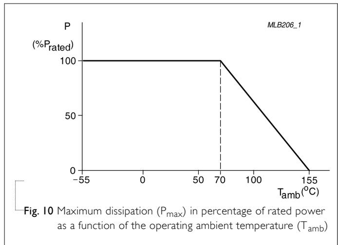
Fig. 10 Maximum dissipation (P<sub>max</sub>) in percentage of rated power as a function of the operating ambient temperature (T<sub>amb</sub>)
