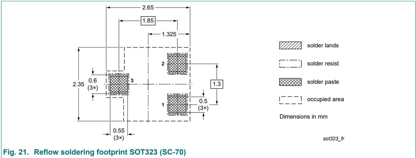
Fig. 21. Reflow soldering footprint SOT323 (SC-70)
