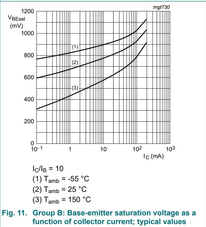
**Fig. 11. Group B: Base-emitter saturation voltage as a function of collector current; typical values**
