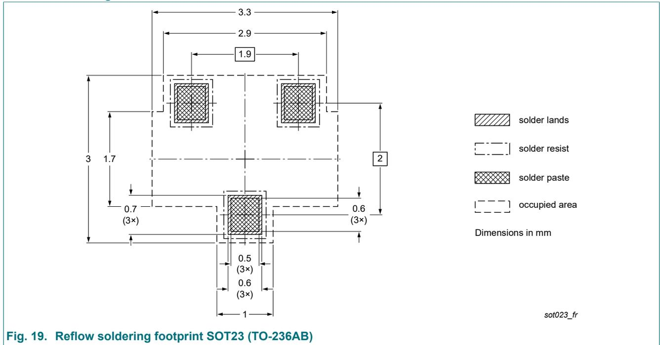
Fig. 19. Reflow soldering footprint SOT23 (TO-236AB)
