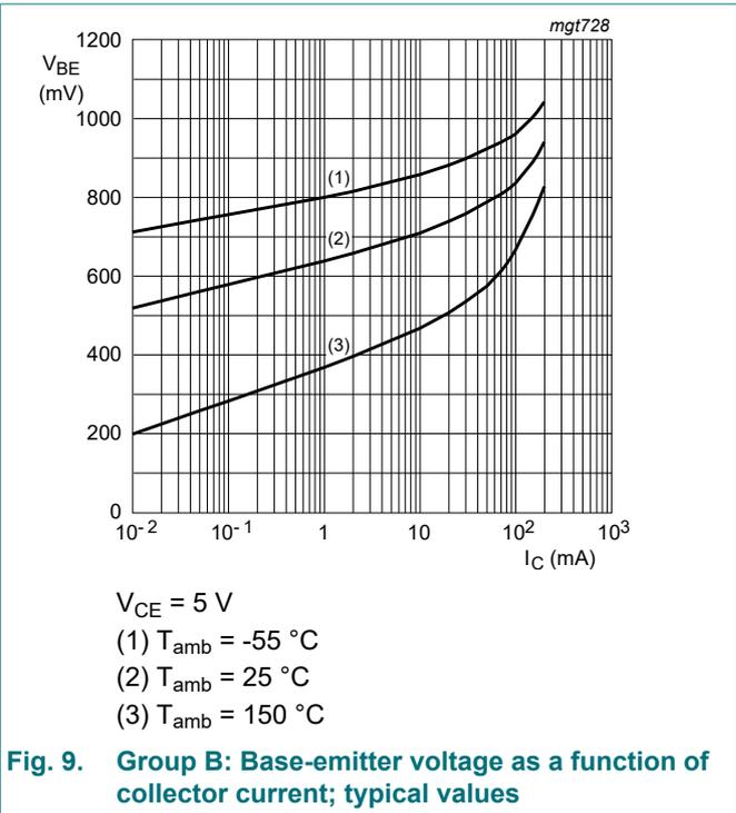
**Fig. 9. Group B: Base-emitter voltage as a function of collector current; typical values**
