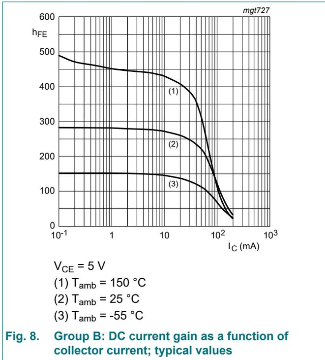
**Fig. 8. Group B: DC current gain as a function of collector current; typical values**
