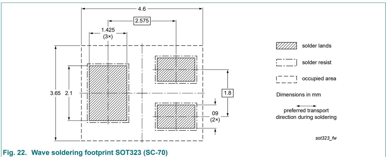
Fig. 22. Wave soldering footprint SOT323 (SC-70)
