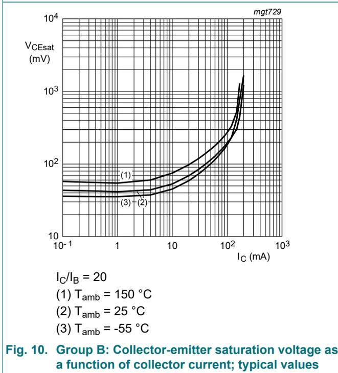
**Fig. 10. Group B: Collector-emitter saturation voltage as a function of collector current; typical values**
