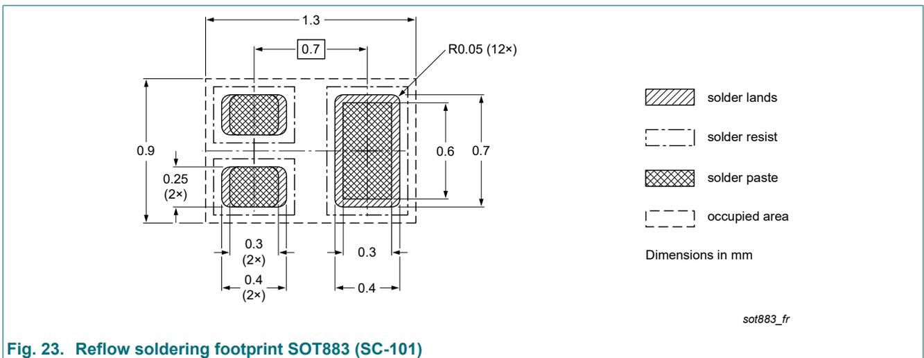
Fig. 23. Reflow soldering footprint SOT883 (SC-101)
