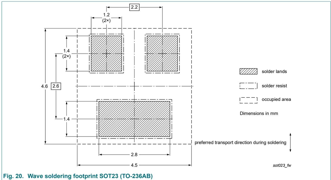
Fig. 20. Wave soldering footprint SOT23 (TO-236AB)
