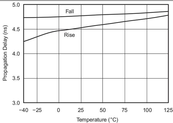
Figure 3. Propagation Delay vs Temperature
