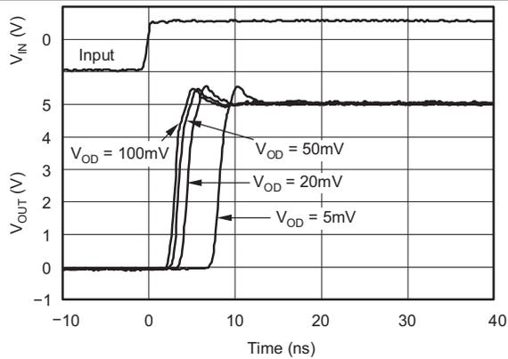
Figure 1. Output Response for Various Overdrive Voltages (Rising)
