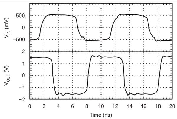
Figure 10. Response to 100-MHz Sine Wave ( $\pm 2.5\text{-V}$  Dual Supply into 50- $\Omega$  Oscilloscope Input)
