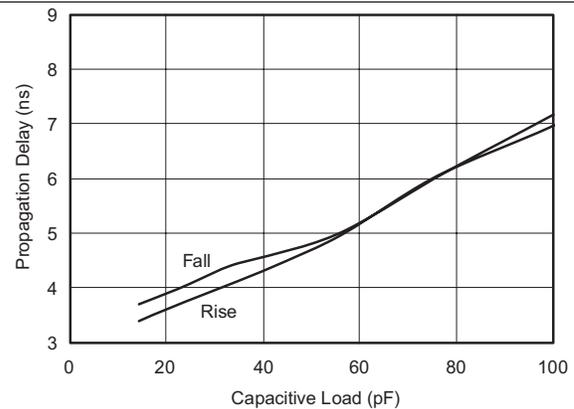
Figure 6. Propagation Delay vs Capacitive Load
