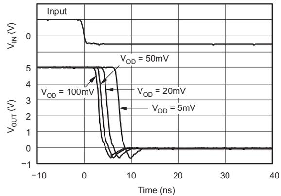
Figure 2. Output Response for Various Overdrive Voltages (Falling)
