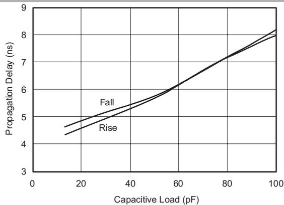
Figure 5. Propagation Delay vs Capacitive Load
