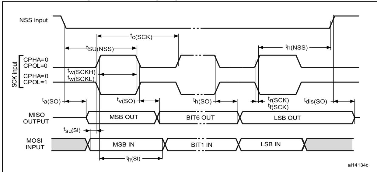
Figure 26. SPI timing diagram - slave mode and CPHA = 1
