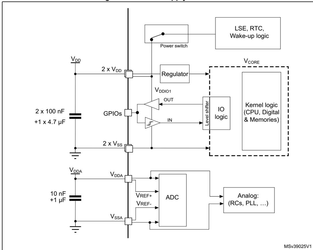
**Caution:** Each power supply pair ( $V_{DD}/V_{SS}$ ,  $V_{DDA}/V_{SSA}$  etc.) must be decoupled with filtering ceramic capacitors as shown above. These capacitors must be placed as close as possible to, or below, the appropriate pins on the underside of the PCB to ensure the good functionality of the device.
