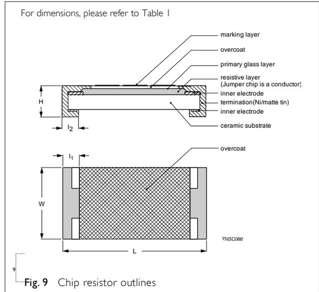
Fig. 9 Chip resistor outlines
