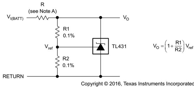
A. R must provide cathode current  $\geq 1$  mA to the TL431-Q1 at minimum  $V_{I(BATT)}$ .
