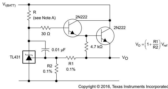
A. R must provide cathode current  $\geq 1$  mA to the TL431-Q1 at minimum  $V_{I(BATT)}$ .
