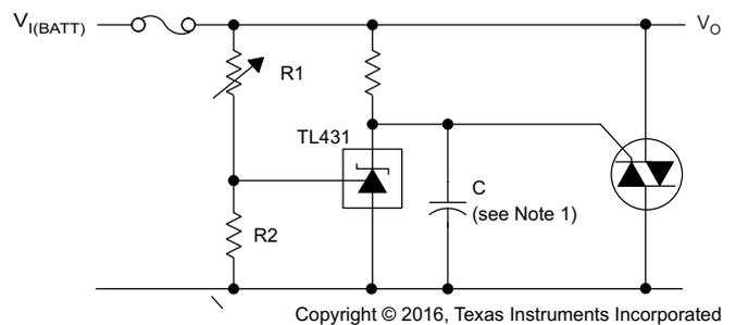
(1) See Figure 12 and Figure 13 to determine allowable values for C.
