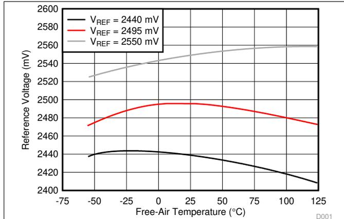
Data is for devices having the indicated value of  $V_{REF}$  at  $I_{KA} = 10$  mA,  $T_A = 25^\circ\text{C}$ .
