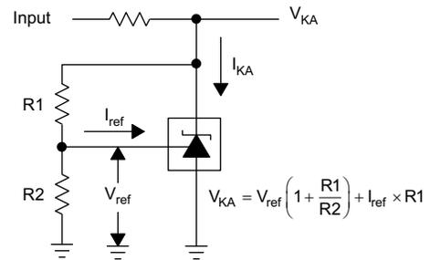
Figure 21. Test Circuit for  $V_{KA} > V_{REF}$
