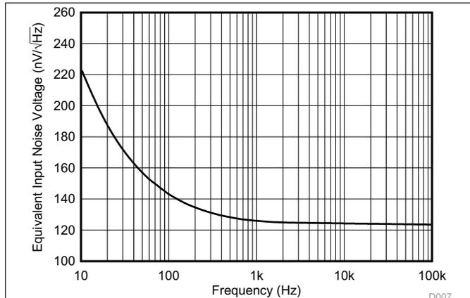
Figure 7. Equivalent Input Noise Voltage vs Frequency
