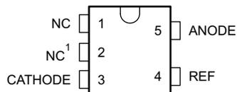
(1) Pin 2 is connected internally to ANODE (die substrate) and must be left floating or connected to ANODE.
