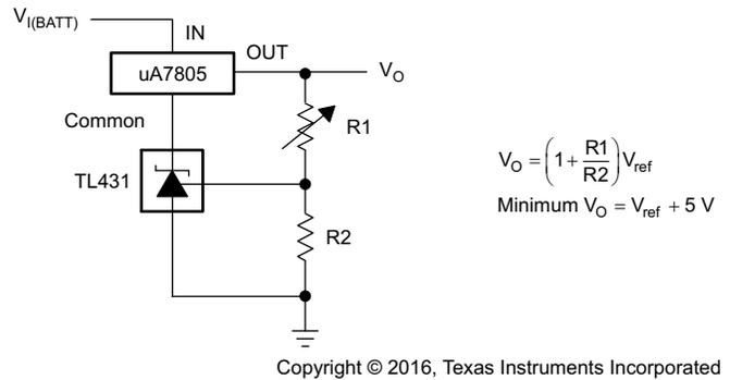
**Figure 31. Output Control of a Three-Terminal Fixed Regulator**
