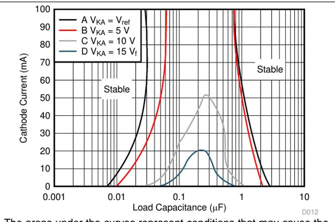
The areas under the curves represent conditions that may cause the device to oscillate. For curves B, C, and D, R2 and V<sub>REF</sub> were adjusted to establish the initial V<sub>KA</sub> and I<sub>KA</sub> conditions with C<sub>L</sub> = 0. V<sub>BATT</sub> and C<sub>L</sub> then were adjusted to determine the ranges of stability (see Figure 18 and Figure 19 for test circuits).
