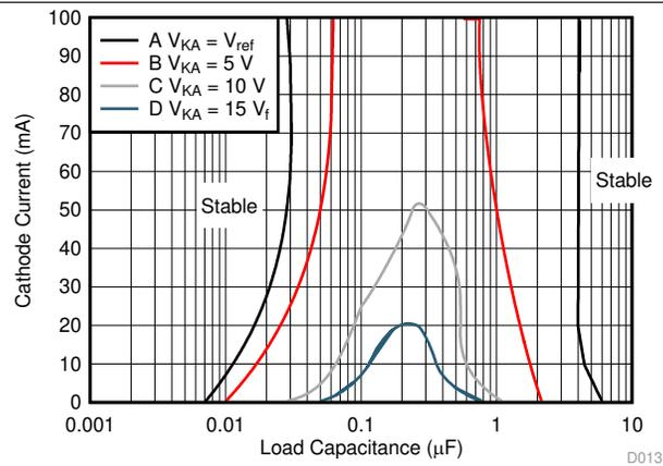
The areas under the curves represent conditions that may cause the device to oscillate. For curves B, C, and D,  $R_2$  and  $V_{REF}$  were adjusted to establish the initial  $V_{KA}$  and  $I_{KA}$  conditions with  $C_L = 0$ .  $V_{BATT}$  and  $C_L$  then were adjusted to determine the ranges of stability (see [Figure 18](#) and [Figure 19](#) for test circuits).
