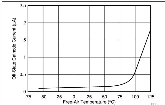
Figure 5. OFF-State Cathode Current vs Free-air Temperature
