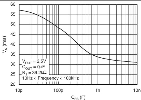
Figure 25. TPS73601 RMS Noise Voltage vs  $C_{FB}$
