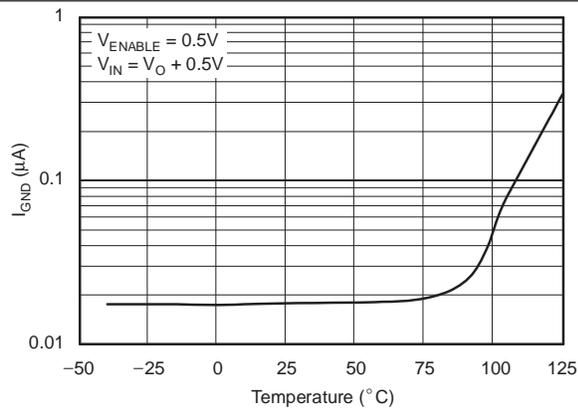
Figure 9. Ground Pin Current In Shutdown vs Temperature
