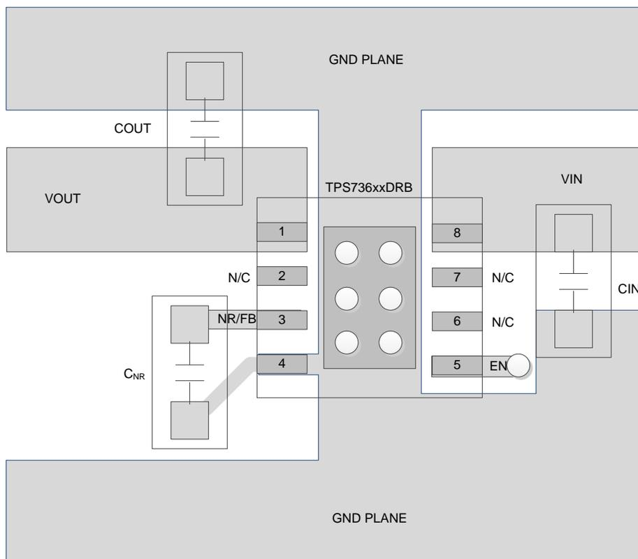
**Figure 37. Fixed Output Voltage Option Layout (DRB Package)**
