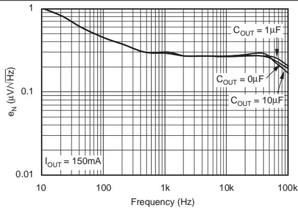
Figure 15. Noise Spectral Density  $c_{NR} = 0\ \mu\text{F}$
