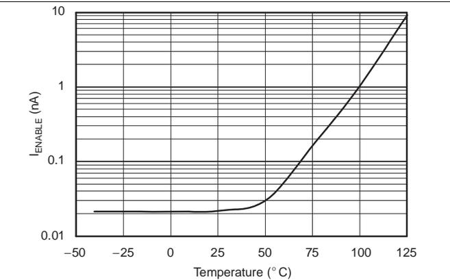
Figure 24.  $I_{ENABLE}$  vs Temperature
