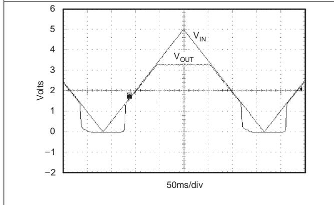
Figure 23. TPS73633 Power Up / Power Down
