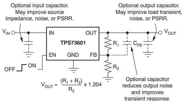
Figure 32. Typical Application Circuit for Adjustable-Voltage Version
