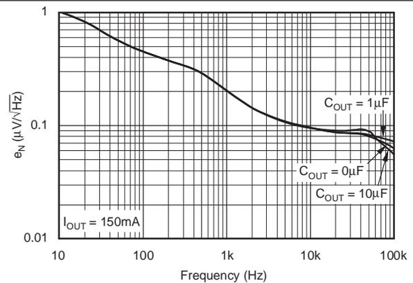
Figure 16. Noise Spectral Density  $c_{NR} = 0.01\ \mu\text{F}$
