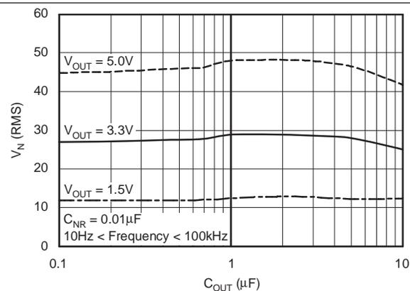
Figure 17. RMS Noise Voltage vs  $C_{OUT}$
