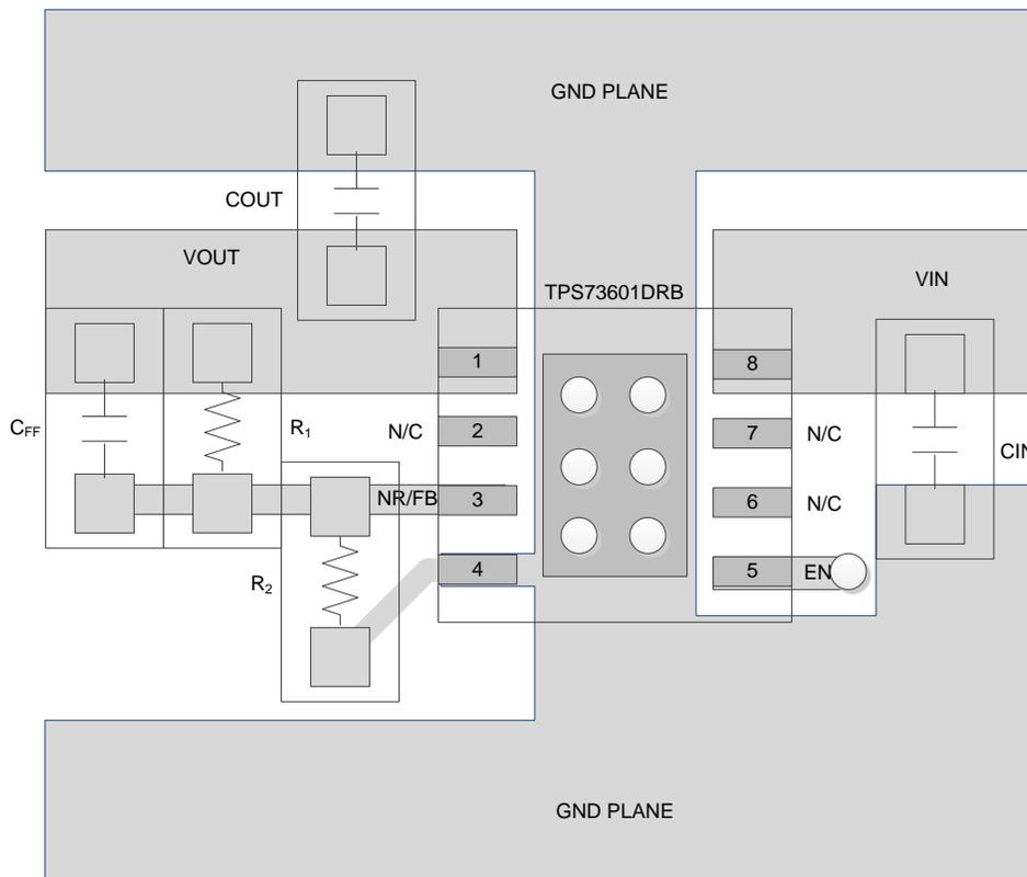
Figure 38. Adjustable Output Voltage Option Layout (DRB Package)
