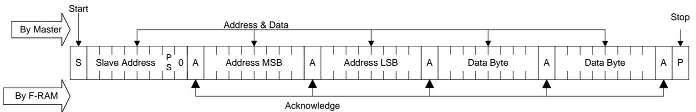
Figure 10. Hs-mode Byte Write
