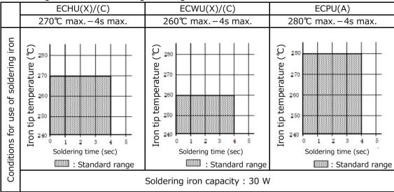
\* Soldering conditions when using soldering iron.
