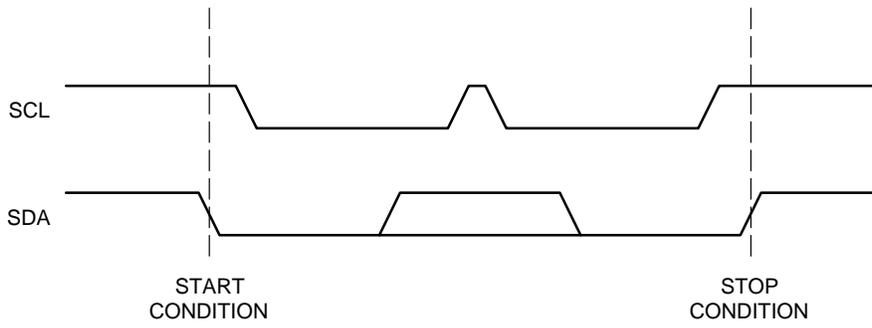
Figure 2. Start/Stop Timing
