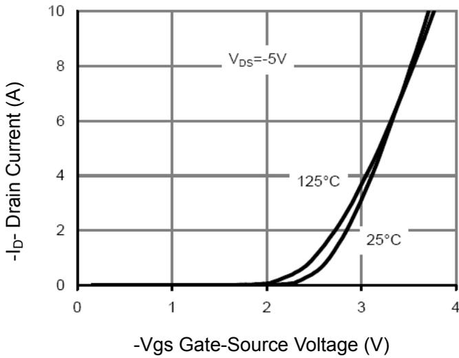
Figure 7 Transfer Characteristics
