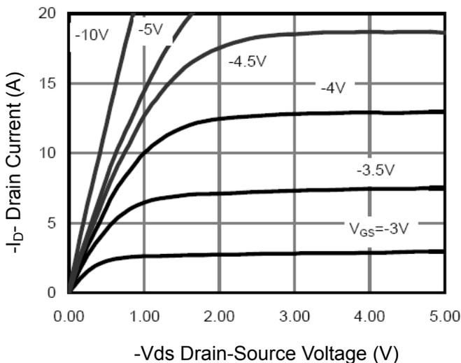
Figure 5 Output Characteristics
