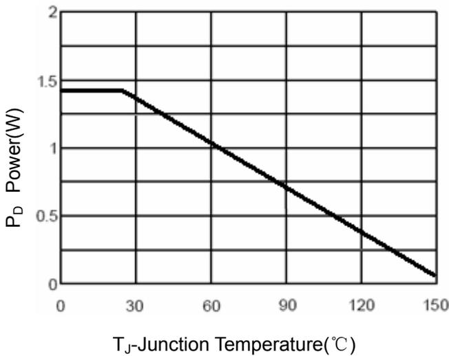
Figure 3 Power Dissipation
