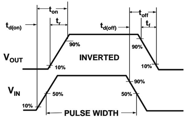
Figure 2: Switching Waveforms
