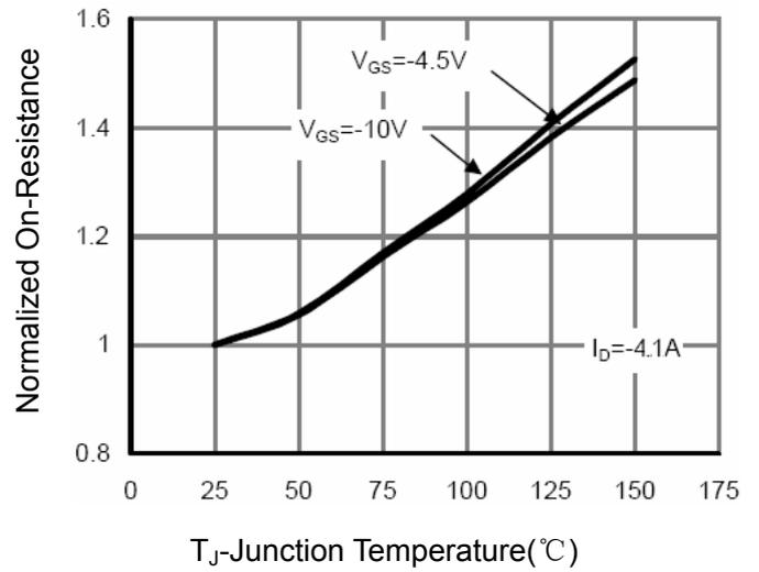
Figure 8 Drain-Source On-Resistance
