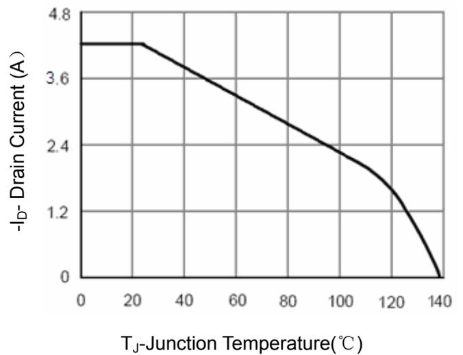
Figure 4 Drain Current
