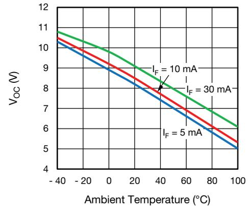
Fig. 4 - Output Open Circuit Voltage vs. Ambient Temperature
