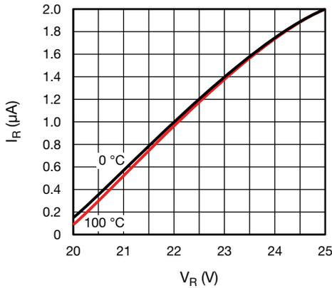
Fig. 6 - LED Reverse Current vs. Reverse Voltage
