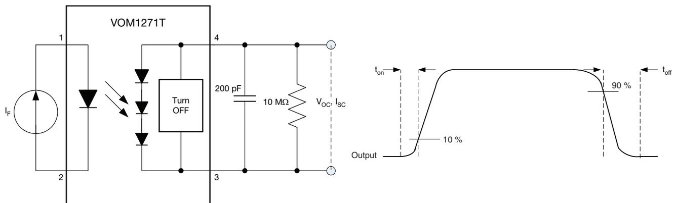
Fig. 1 -  $t_{on}$ ,  $t_{off}$  Test Circuit and Waveforms
