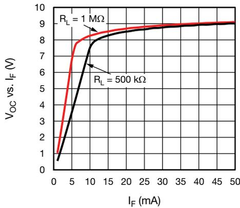
Fig. 2 - Output Open Circuit Voltage vs. LED Current
