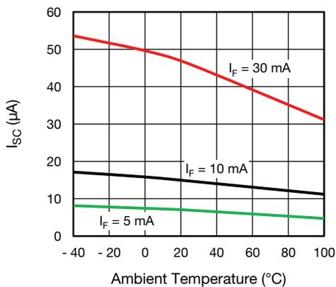
Fig. 3 - Output Short-Circuit Current vs. Ambient Temperature
