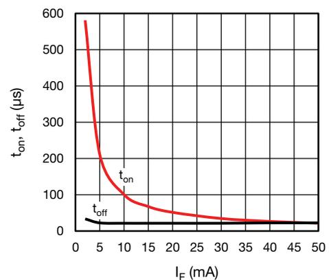
Fig. 5 -  $t_{on}$ ,  $t_{off}$  vs. LED Current
