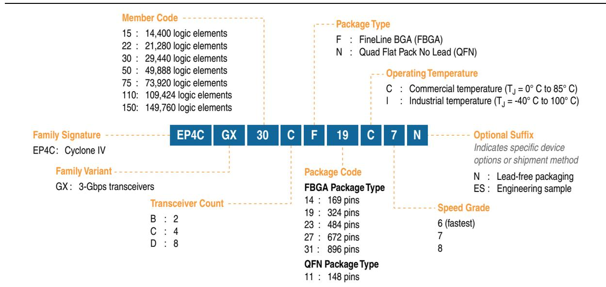
Figure 1-3 shows the ordering codes for Cyclone IV E devices.
