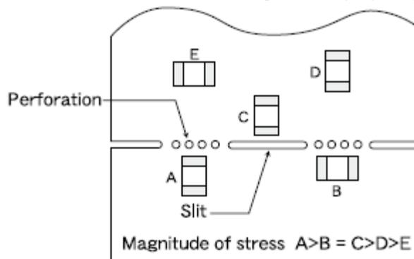
1-3. When PCB is split, the amount of mechanical stress on the capacitors can vary according to the method used. The following methods are listed in order from least stressful to most stressful: push-back, slit, V-grooving, and perforation. Thus, please consider the PCB, split methods as well as chip location.
