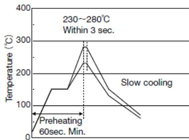
【Recommended condition for Pb-free soldering】
