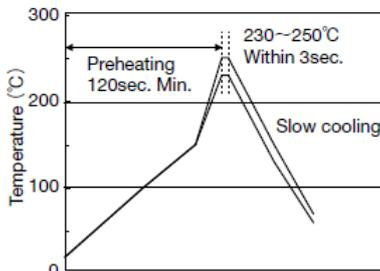
【Recommended condition for Pb-free soldering】
