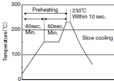
【Recommended condition for Pb-free soldering】
