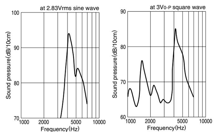
\* The frequency characteristic changes depending on the case shape and the installation method.
