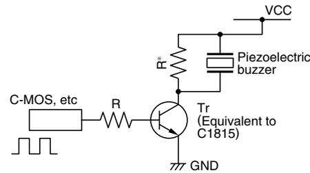
\* Resistor to do charging and discharging to a piezoelectric element (Value of about 1k $\Omega$  is good efficiency).
