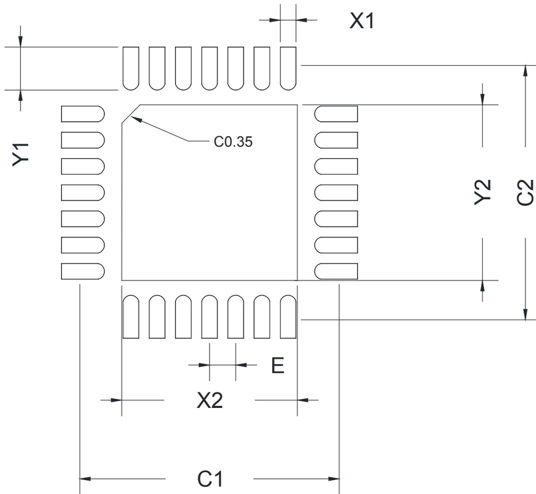
Figure 6.2. QFN28 PCB Land Pattern Drawing
