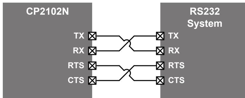
Figure 4.1. Using Hardware Flow Control with the CP2102N
