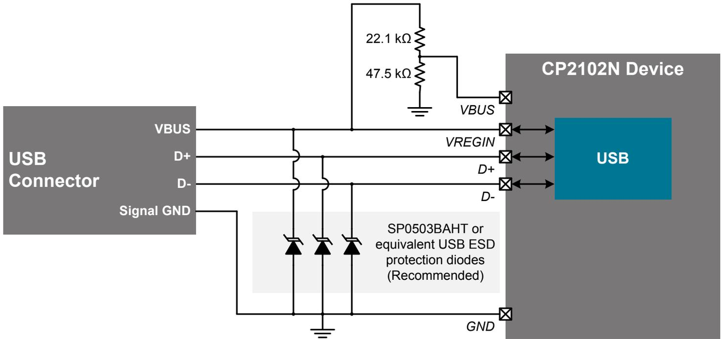
Figure 2.5. Bus-Powered Connection Diagram for USB Pins
