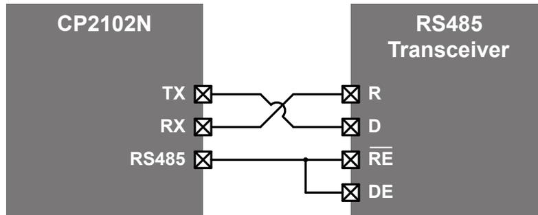
Figure 4.4. Using the CP2102N with a RS485 Transceiver
