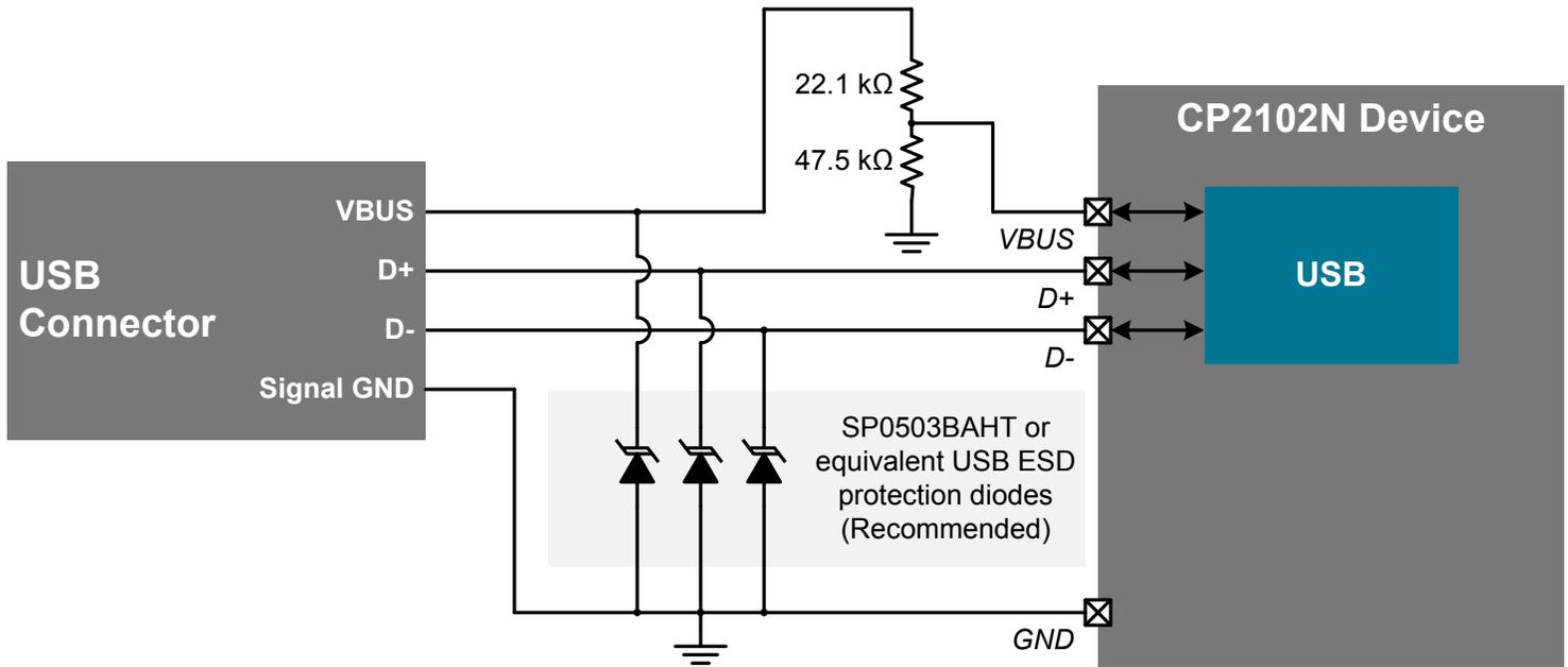
Figure 2.6. Self-Powered Connection Diagram for USB Pins
