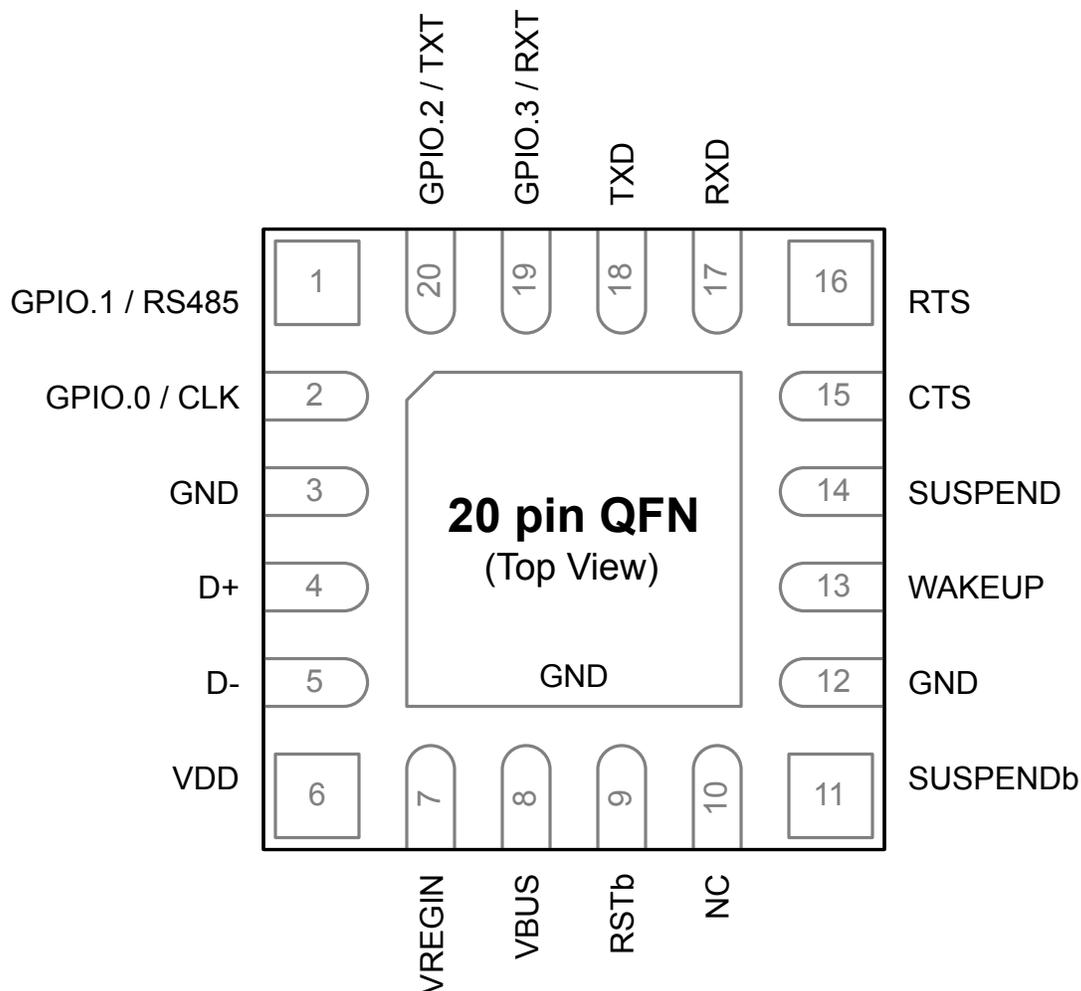
Figure 5.3. CP2102N QFN20 Pinout
