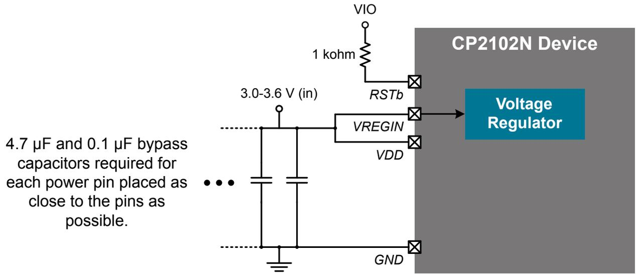
Figure 2.3. Connection Diagram with Voltage Regulator Not Used
