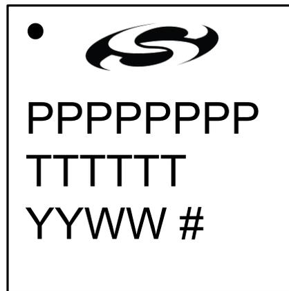
**Figure 6.3. QFN28 Package Marking**
