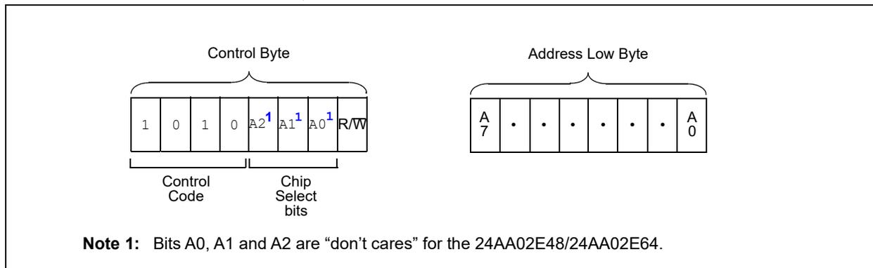
FIGURE 5-1: CONTROL BYTE ALLOCATION
