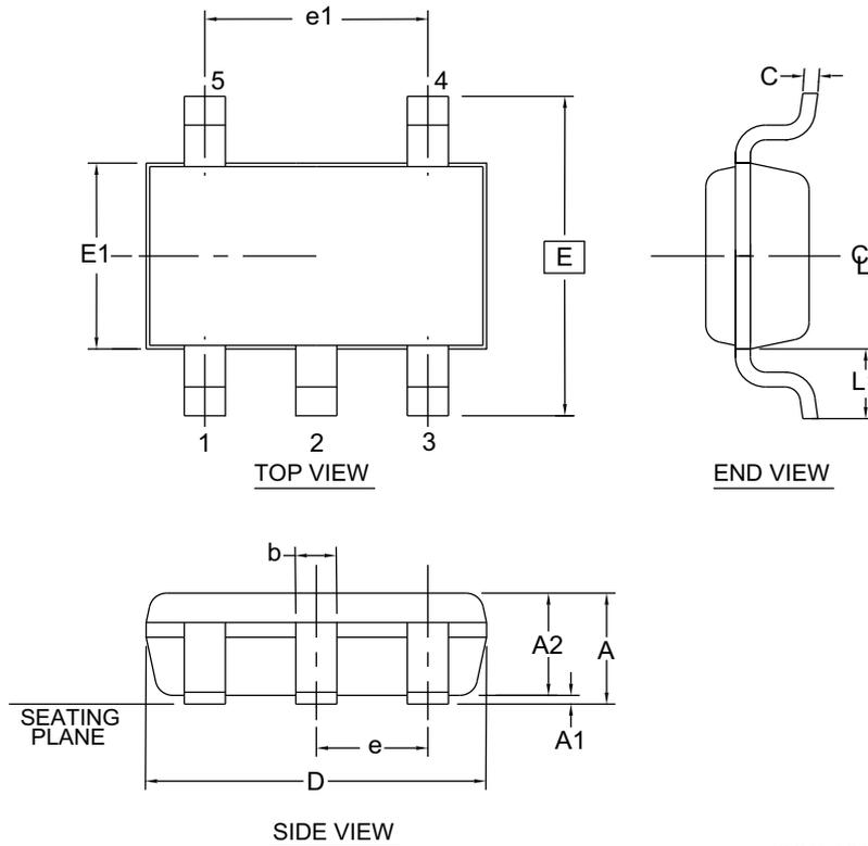
1. Dimension D does not include mold flash, protrusions or gate burrs. Mold flash, protrusions or gate burrs shall not exceed 0.15 mm per end. Dimension E1 does not include interlead flash or protrusion. Interlead flash or protrusion shall not exceed 0.15 mm per side.
