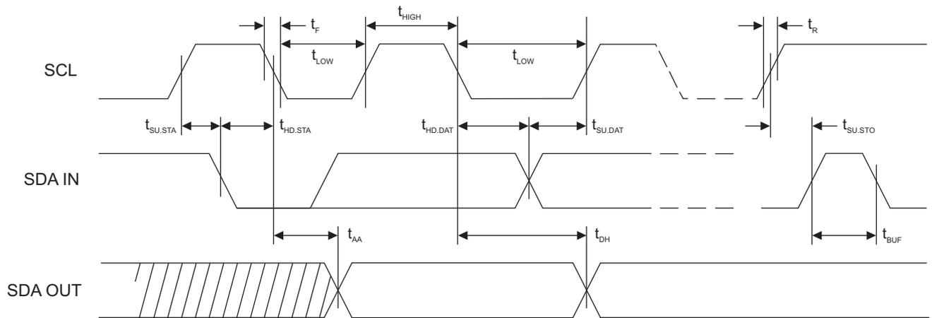
**Figure 6-6. Write Cycle Timing**
