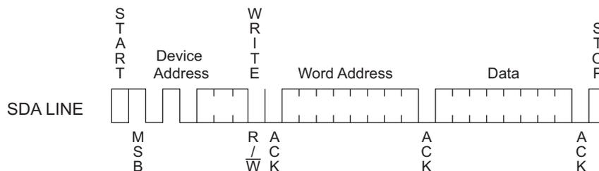
**Page Write:** The 1-Kbit and 2-Kbit EEPROM are capable of an 8-byte Page Write.
