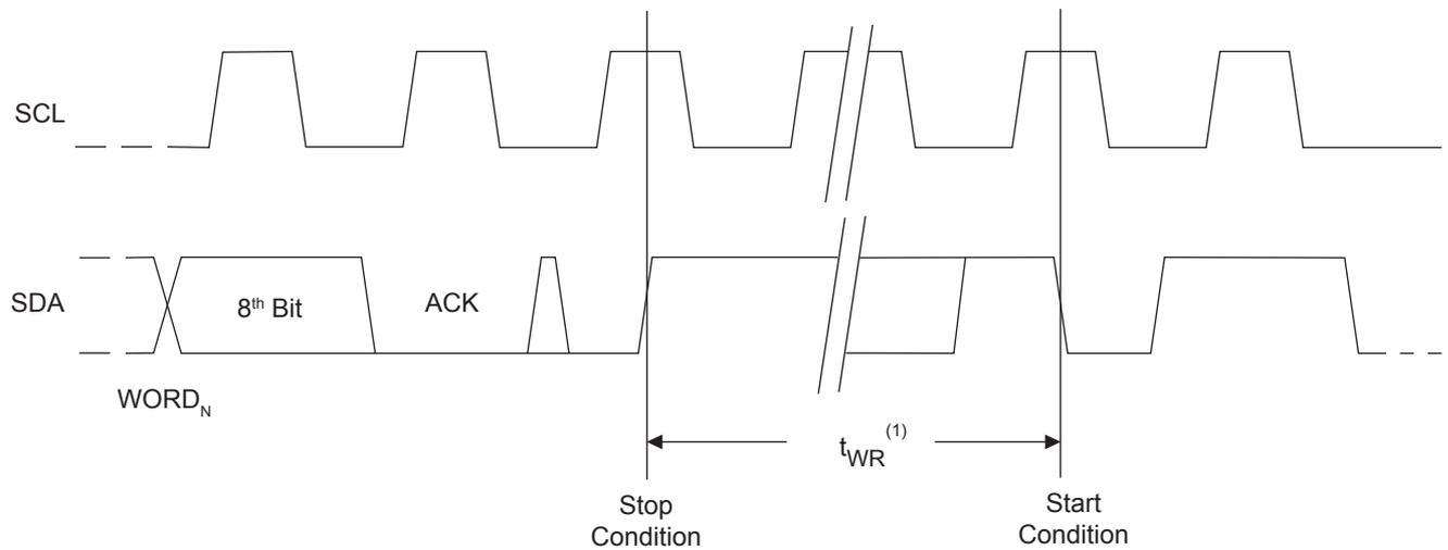
Note: 1. The write cycle time  $t_{WR}$  is the time from a valid Stop condition of a write sequence to the end of the internal clear/write cycle.
