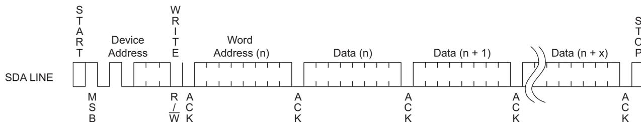
**Acknowledge Polling:** Once the internally timed write cycle has started and the EEPROM inputs are disabled, acknowledge polling can be initiated. This involves sending a Start condition followed by the device address word. The read/write bit is representative of the operation desired. Only if the internal write cycle has completed will the EEPROM respond with a zero allowing the read or write sequence to continue.
