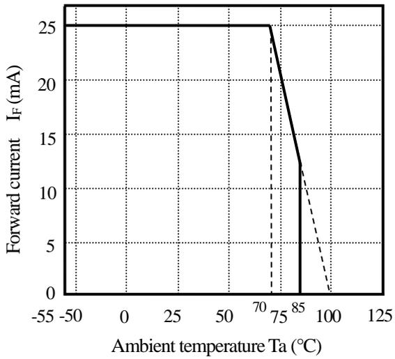
(Fig. 4) Input power dissipation vs. Ambient temperature
