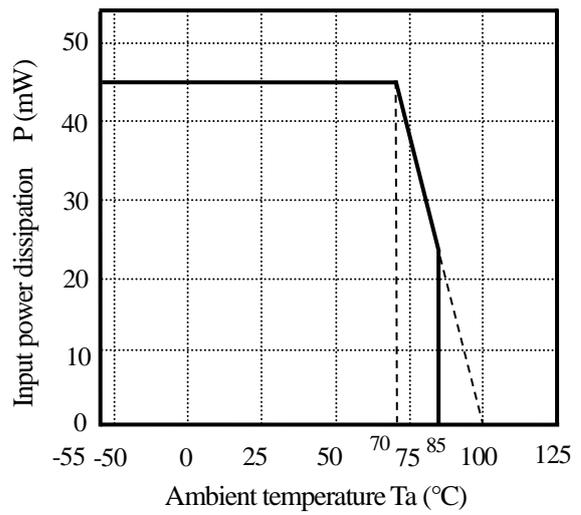
(Fig. 5) Output power dissipation vs. Ambient temperature
