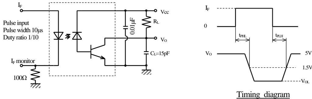
Fig. 2  $CM_H, CM_L$  test circuit
