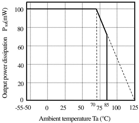
(Note) The total power dissipation ( $P_{tot}$ ) decreases of the ratio of 1.8mW/°C at ambient temperature 70°C or more. (Refer to Fig. 5)
