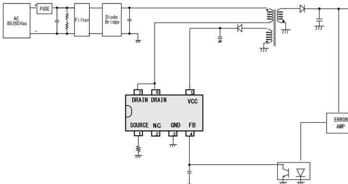
Figure 1. Application circuit
