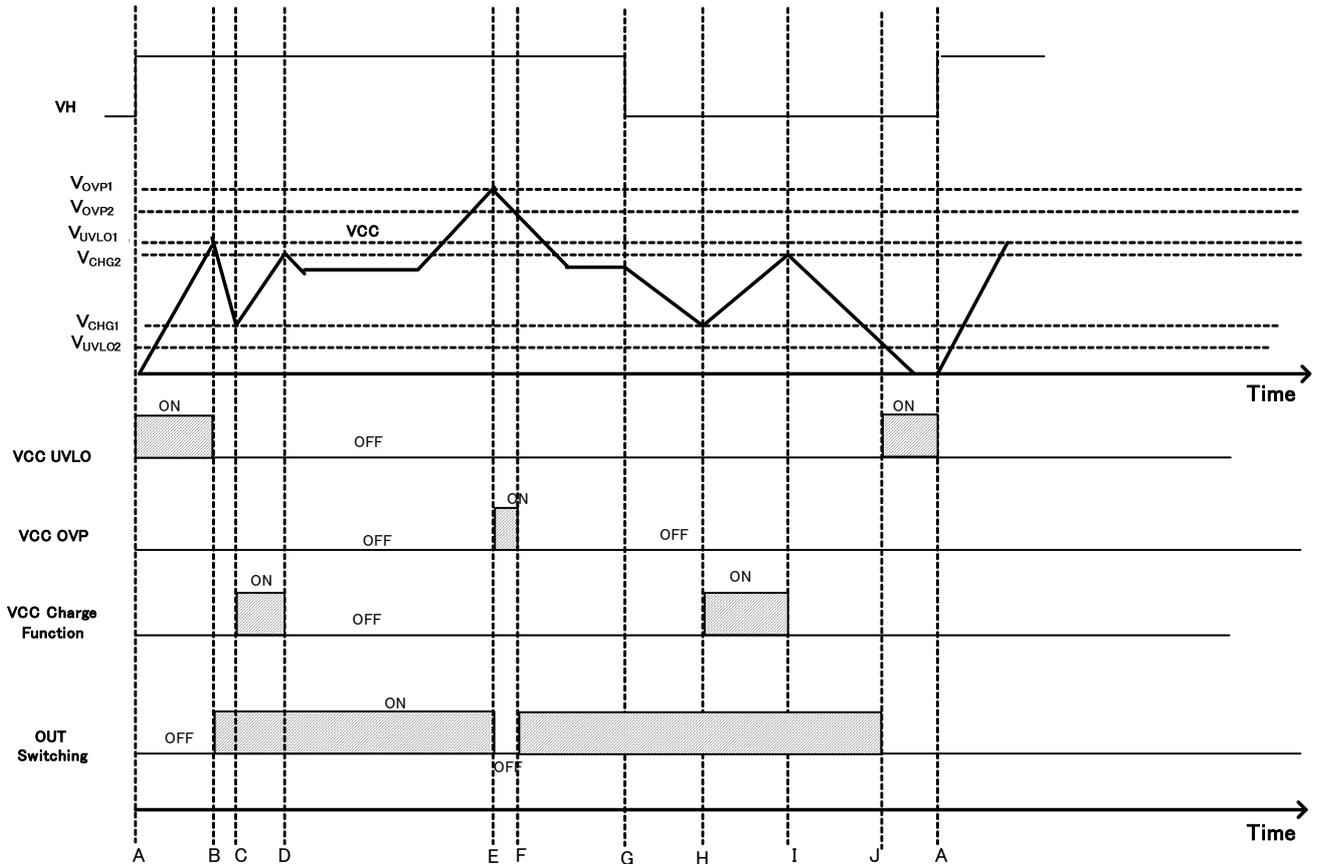
Figure 8. VCC UVLO / OVP Timing Chart
