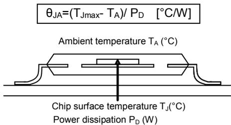
Figure 6. Thermal resistance
