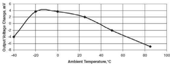
Fig. 13: Line Regulation vs Temperature
