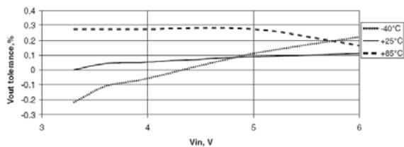
Fig. 15: Line Regulation over Temperature
