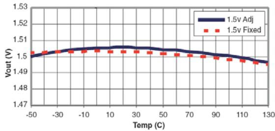
Fig. 9:  $V_{IN}=3.0V$ ,  $I_{OUT}=10mA$
