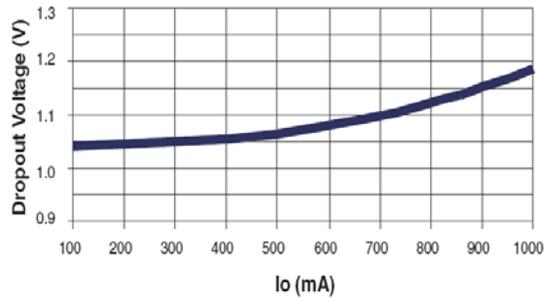
Fig. 5: Dropout Voltage vs Output Current
