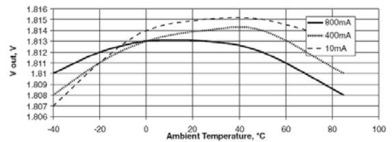
Fig. 14: Output Voltage vs Temperature
