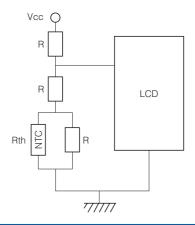
Temperature Compensation (RF circuit)
