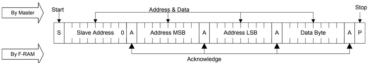
Figure 8. Multi-Byte Write
