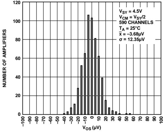
Figure 87. Input Offset Voltage Distribution,  $V_{SY} = 4.5\text{ V}$
