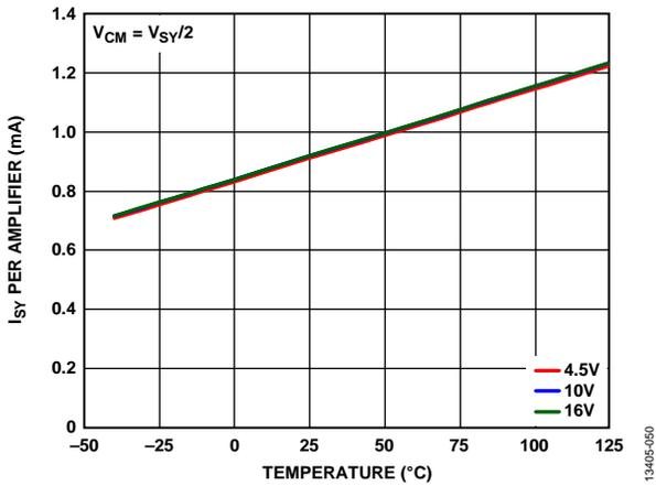
Figure 53. Supply Current ( $I_{sv}$ ) per Amplifier vs. Temperature
