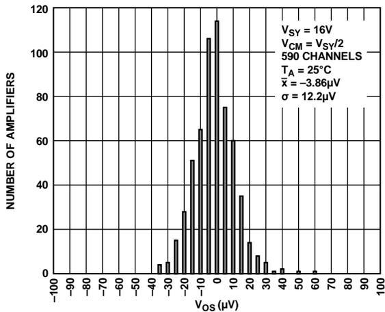
Figure 89. Input Offset Voltage Distribution,  $V_{SY} = 16\text{ V}$
