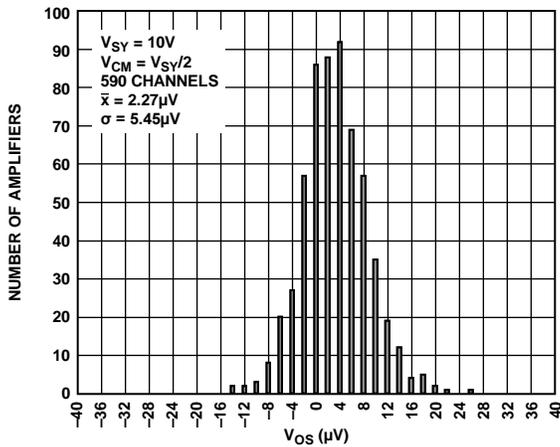
Figure 5. Input Offset Voltage Distribution, V<sub>Sy</sub> = 10 V
