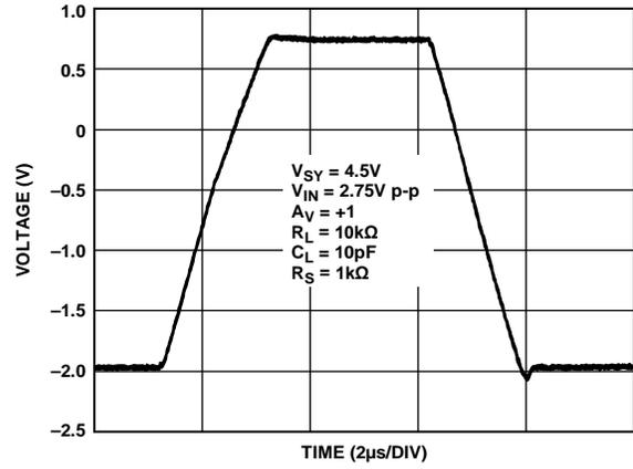
Figure 64. Large Signal Transient Response,  $V_{SY} = 4.5 V$
