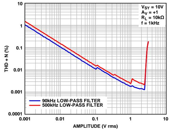
Figure 83. THD + N vs. Amplitude,  $V_{SY} = 10V$
