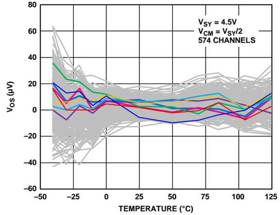
Figure 7. Input Offset Voltage (V<sub>Os</sub>) vs. Temperature, V<sub>Sy</sub> = 4.5 V
