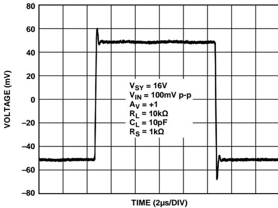
Figure 63. Small Signal Transient Response,  $V_{SY} = 16 V$
