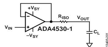
Figure 101. Stability Compensation with Isolating Resistor,  $R_{ISO}$
