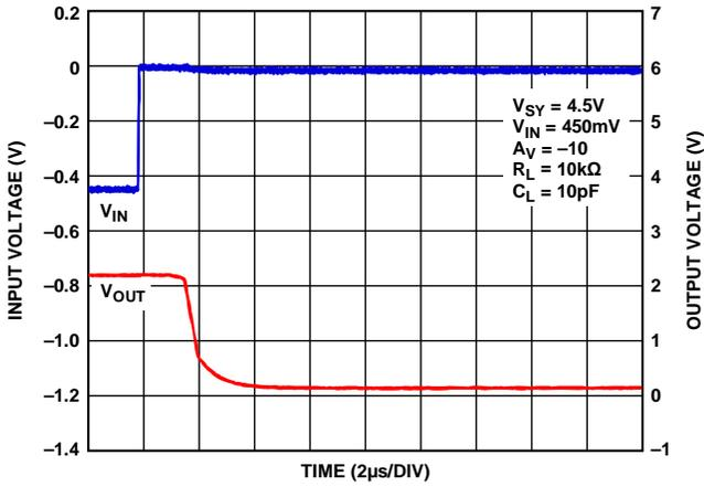
Figure 67. Positive Overload Recovery,  $V_{SY} = 4.5V$
