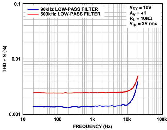
Figure 80. THD + N vs. Frequency,  $V_{SY} = 10V$
