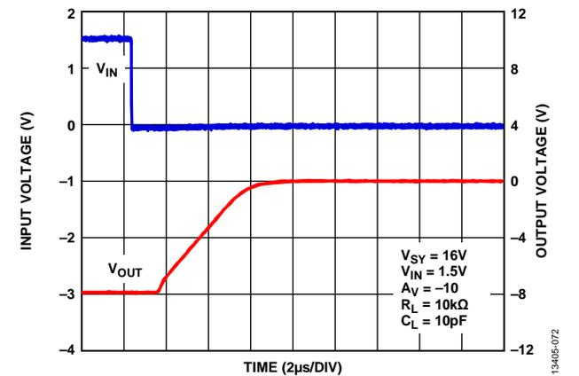
Figure 72. Negative Overload Recovery,  $V_{SY} = 16V$
