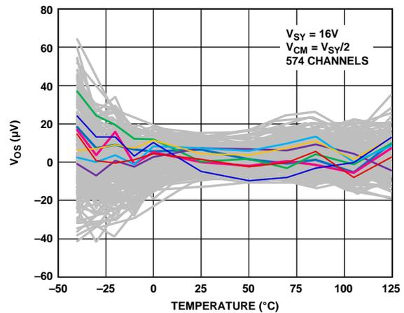
Figure 9. Input Offset Voltage (V<sub>Os</sub>) vs. Temperature, V<sub>Sy</sub> = 16 V
