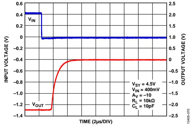
Figure 70. Negative Overload Recovery,  $V_{SY} = 4.5V$
