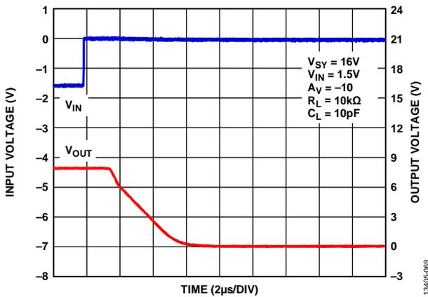
Figure 69. Positive Overload Recovery,  $V_{SY} = 16V$
