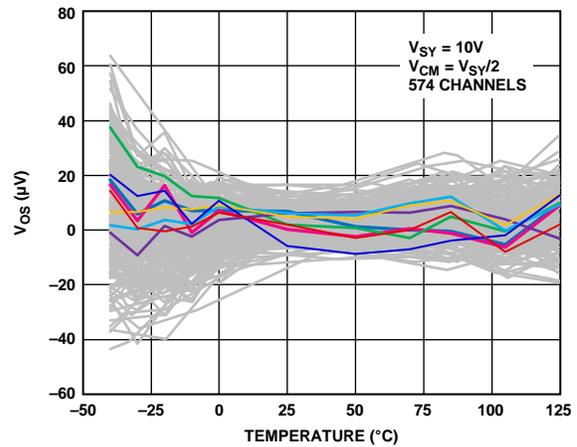
Figure 8. Input Offset Voltage (V<sub>Os</sub>) vs. Temperature, V<sub>Sy</sub> = 10 V
