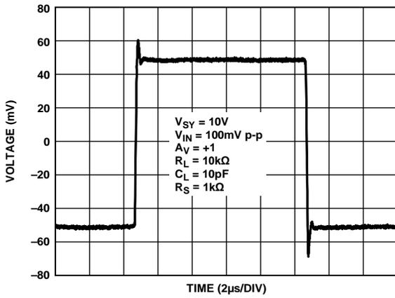
Figure 62. Small Signal Transient Response,  $V_{SY} = 10 V$
