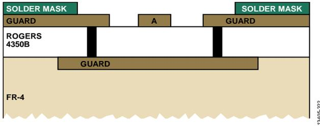
Figure 123. Layout Cross Section with Guard Plane
