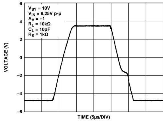
Figure 65. Large Signal Transient Response,  $V_{SY} = 10 V$
