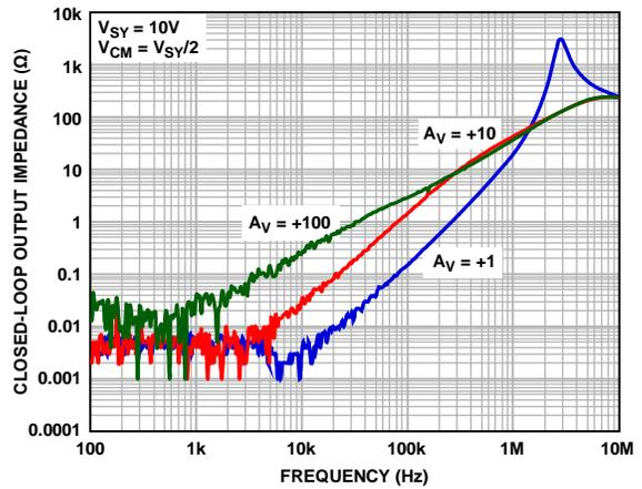
Figure 59. Closed-Loop Output Impedance vs. Frequency
