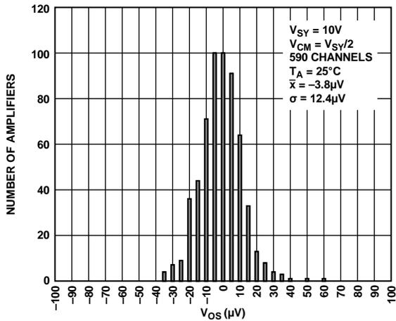
Figure 88. Input Offset Voltage Distribution,  $V_{SY} = 10\text{ V}$
