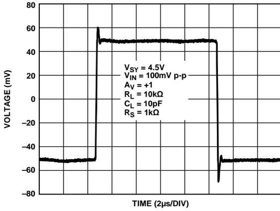
Figure 61. Small Signal Transient Response,  $V_{SY} = 4.5 V$
