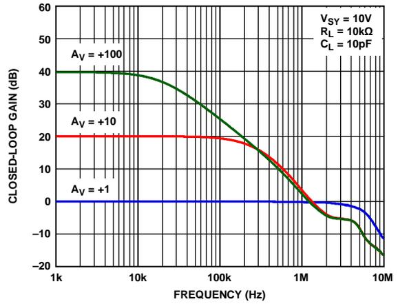
Figure 58. Closed-Loop Gain vs. Frequency
