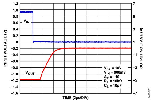
Figure 71. Negative Overload Recovery,  $V_{SY} = 10V$
