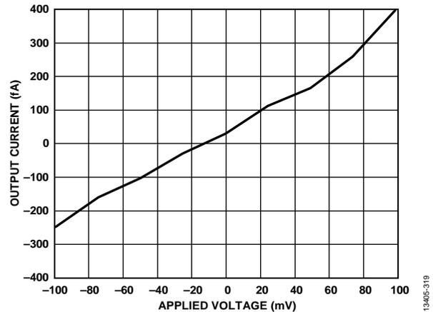
Figure 114. Current to Voltage Response of RMA Contaminated Insulation
