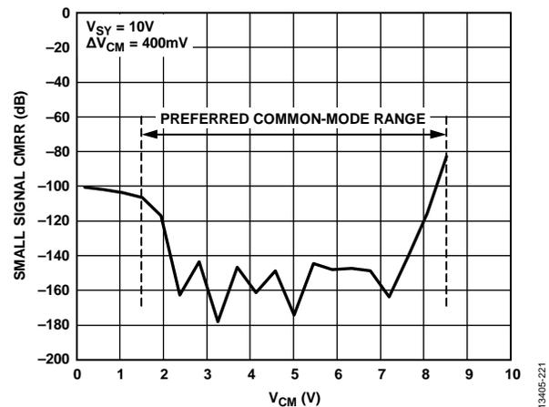
Figure 21. Small Signal CMRR vs. Common-Mode Voltage ( $V_{CM}$ )
