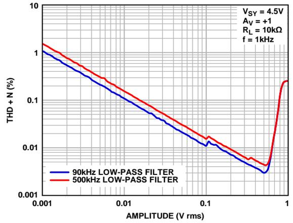
Figure 82. THD + N vs. Amplitude,  $V_{SY} = 4.5V$
