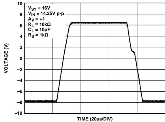
Figure 66. Large Signal Transient Response,  $V_{SY} = 16 V$
