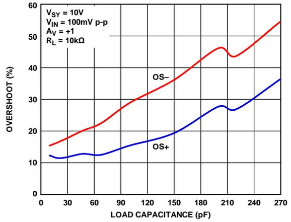
Figure 60. Small Signal Overshoot vs. Load Capacitance
