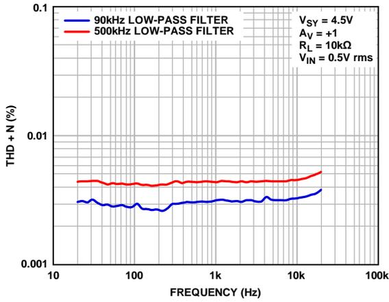
Figure 79. THD + N vs. Frequency,  $V_{SY} = 4.5V$
