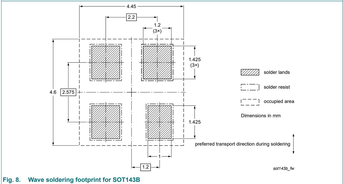
Fig. 8. Wave soldering footprint for SOT143B
