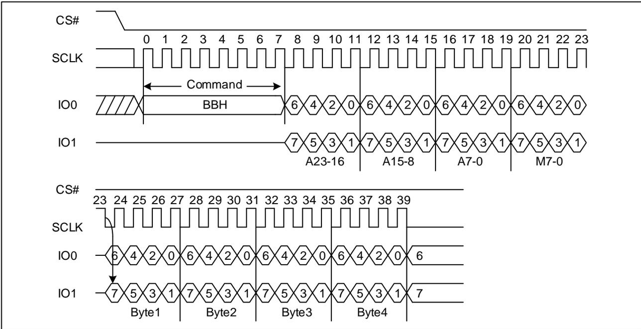
**Figure 13. Dual I/O Fast Read Sequence Diagram ((M5-4) = (1, 0))**
