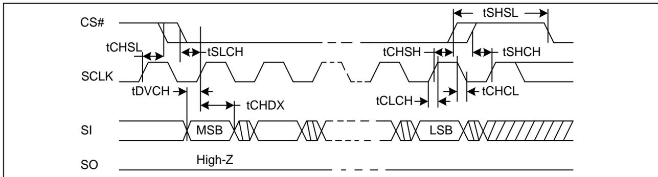
**Figure 40. Output Timing**
