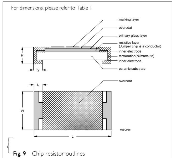
Fig. 9 Chip resistor outlines
