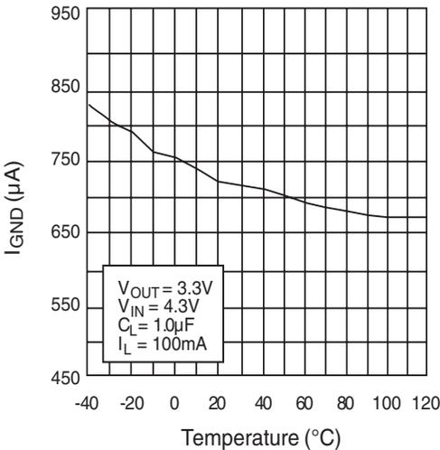
Figure 8. Ground Current vs. Temperature at I<sub>LOAD</sub> = 100mA
