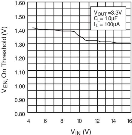
Figure 11. ENABLE Voltage, ON Threshold vs. Input Voltage
