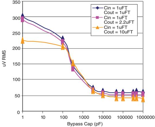
Figure 12. Output Noise vs. Bypass Capacitor Value
