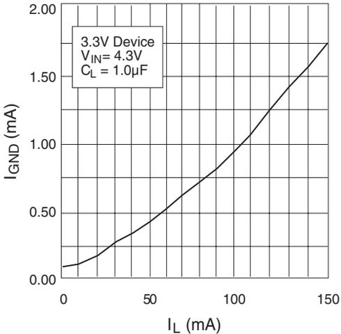
Figure 3. Ground Current vs. Load Current in Dropout
