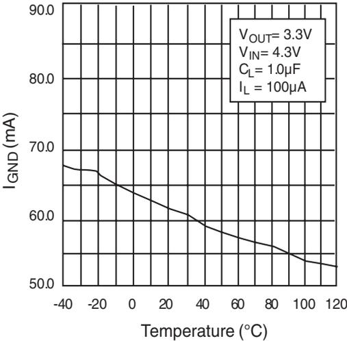
Figure 7. Ground Current vs. Temperature at I<sub>LOAD</sub> = 100µA
