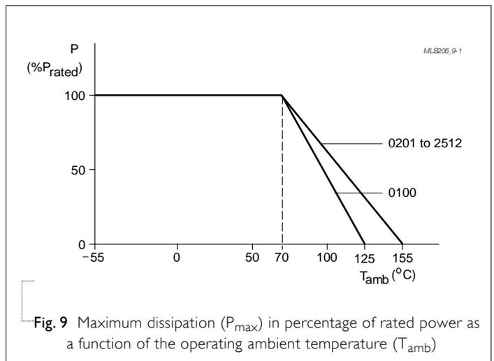
Fig. 9 Maximum dissipation (P<sub>max</sub>) in percentage of rated power as a function of the operating ambient temperature (T<sub>amb</sub>)
