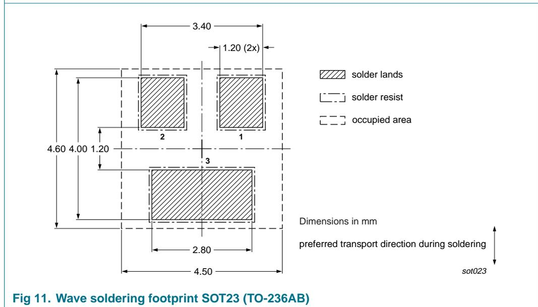
**Fig 11. Wave soldering footprint SOT23 (TO-236AB)**
