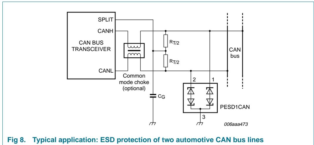
**Fig 8. Typical application: ESD protection of two automotive CAN bus lines**
