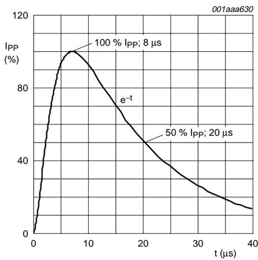
**Fig 1. 8/20 μs pulse waveform according to IEC 61000-4-5**
