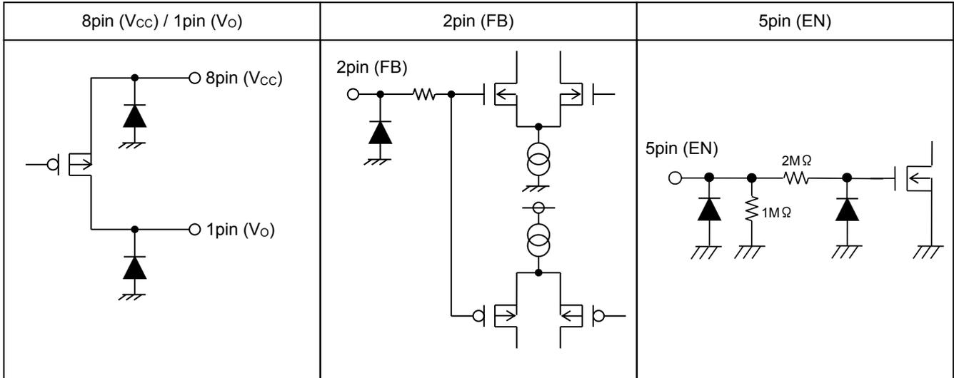
● I/O Equivalent Circuits (Fixed type :BDxxHC5WEFJ)
