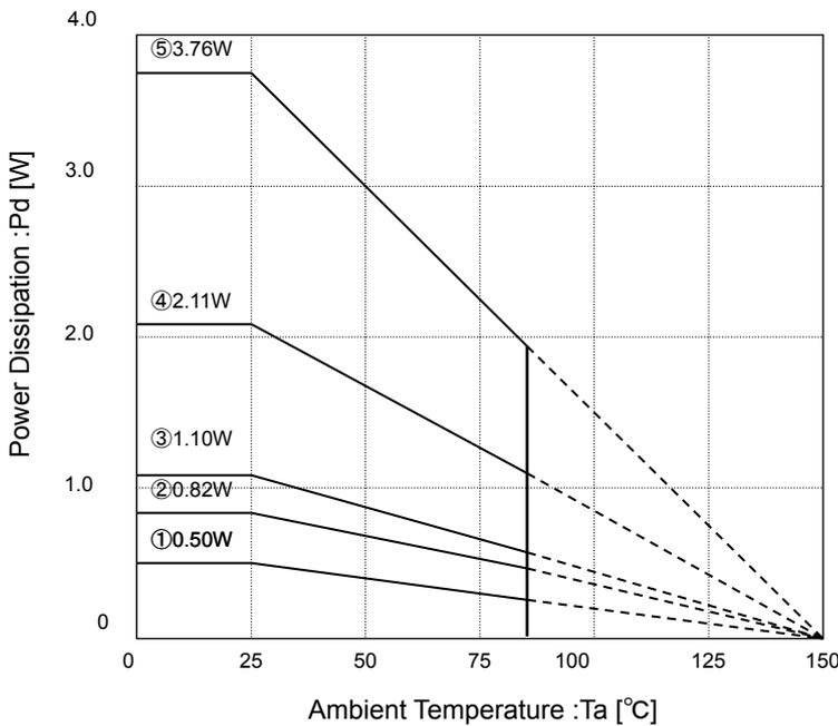
Measurement condition: mounted on a ROHM board,
