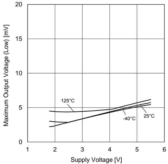
Figure 7. Maximum Output Voltage (Low) vs Supply Voltage ( $R_L=10\text{ k}\Omega$ )
