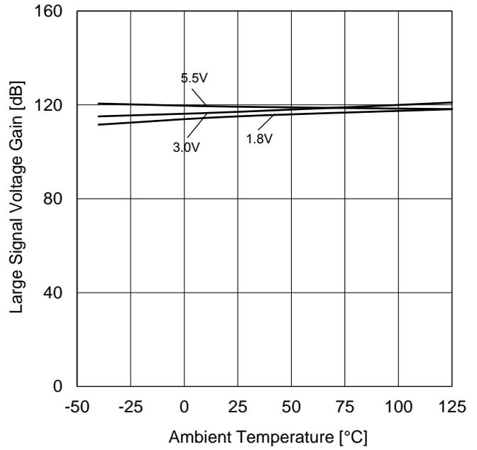
Figure 23. Large Signal Voltage Gain vs Ambient Temperature
