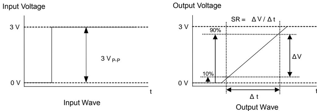
Figure 32. Slew Rate Input and Output Wave
