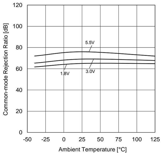
Figure 25. Common-mode Rejection Ratio vs Ambient Temperature
