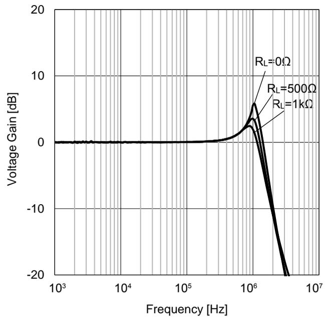
Figure 41. Voltage Gain vs Frequency
