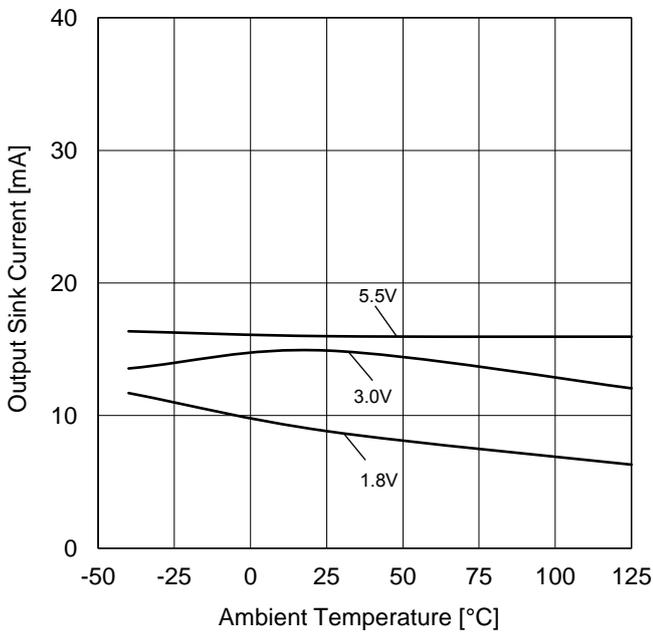
Figure 16. Output Sink Current vs Ambient Temperature (V<sub>OUT</sub>=V<sub>SS</sub>+0.4 V)
