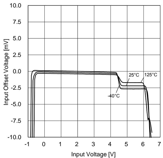
Figure 21. Input Offset Voltage vs Input Voltage ( $V_{DD}=5.5\text{ V}$ )
