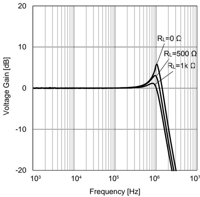
Figure 40. Voltage Gain vs Frequency
