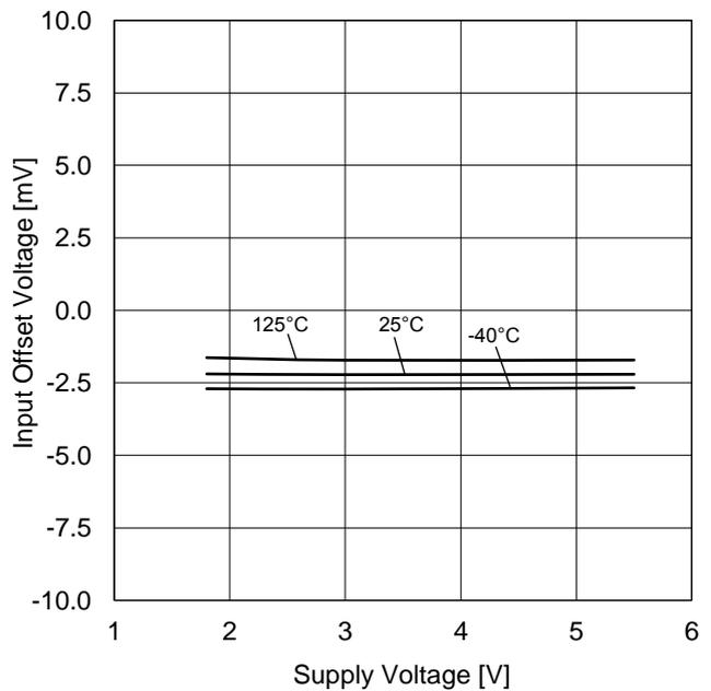
Figure 17. Input Offset Voltage vs Supply Voltage (V<sub>ICM</sub>=V<sub>DD</sub>, E<sub>K</sub>=-V<sub>DD</sub>/2)
