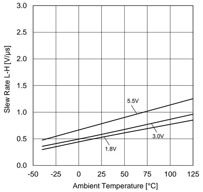
Figure 27. Slew Rate L-H vs Ambient Temperature
