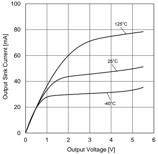
Figure 15. Output Sink Current vs Output Voltage (V<sub>DD</sub>=5.5 V)
