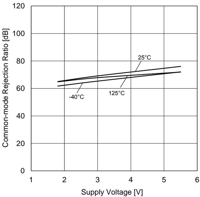
Figure 24. Common-mode Rejection Ratio vs Supply Voltage
