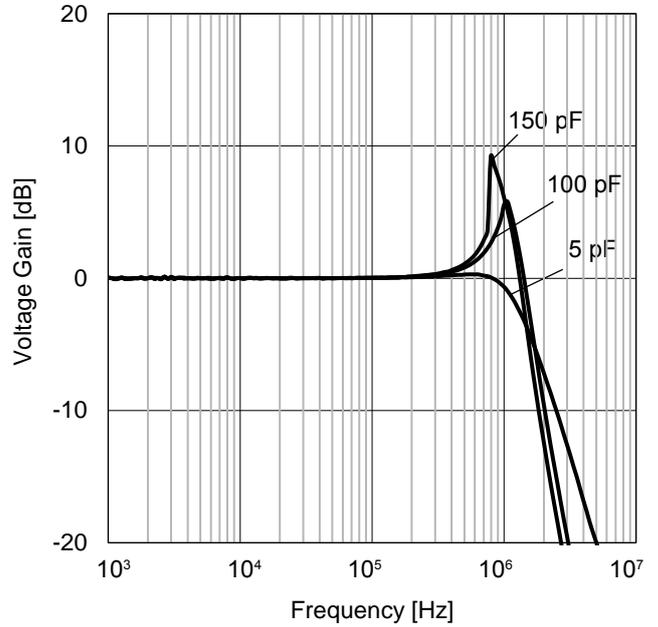
Figure 35. Voltage Gain vs Frequency (V<sub>DD</sub>=3.0 V, G<sub>v</sub>=0 dB)
