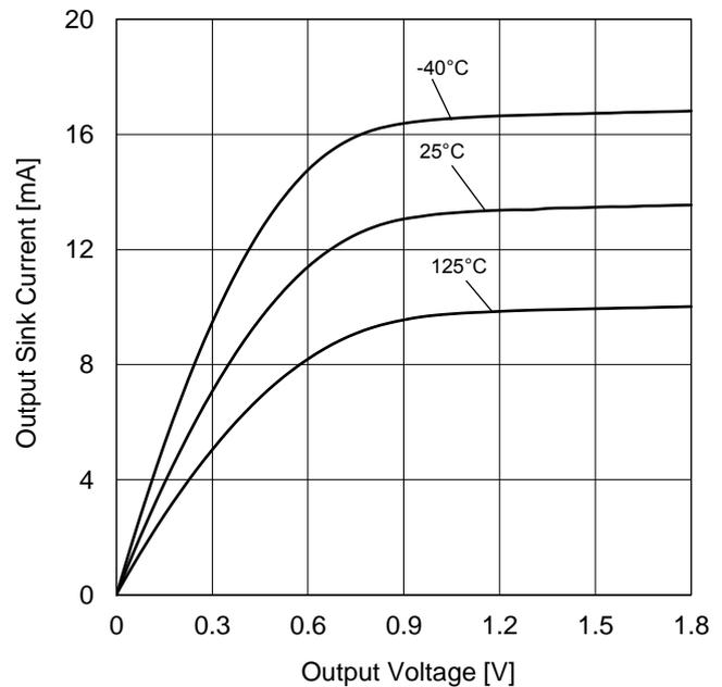
Figure 13. Output Sink Current vs Output Voltage (V<sub>DD</sub>=1.8 V)
