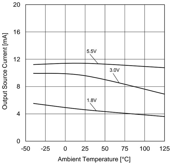
Figure 12. Output Source Current vs Ambient Temperature (V<sub>OUT</sub>=V<sub>DD</sub>-0.4 V)
