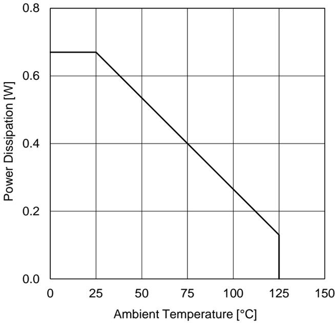
Figure 2. Power Dissipation vs Ambient Temperature (Derating Curve)
