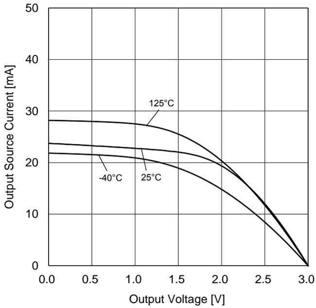
Figure 10. Output Source Current vs Output Voltage (V<sub>DD</sub>=3.0 V)
