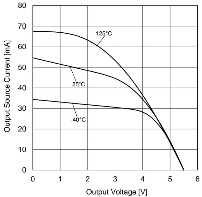
Figure 11. Output Source Current vs Output Voltage (V<sub>DD</sub>=5.5 V)
