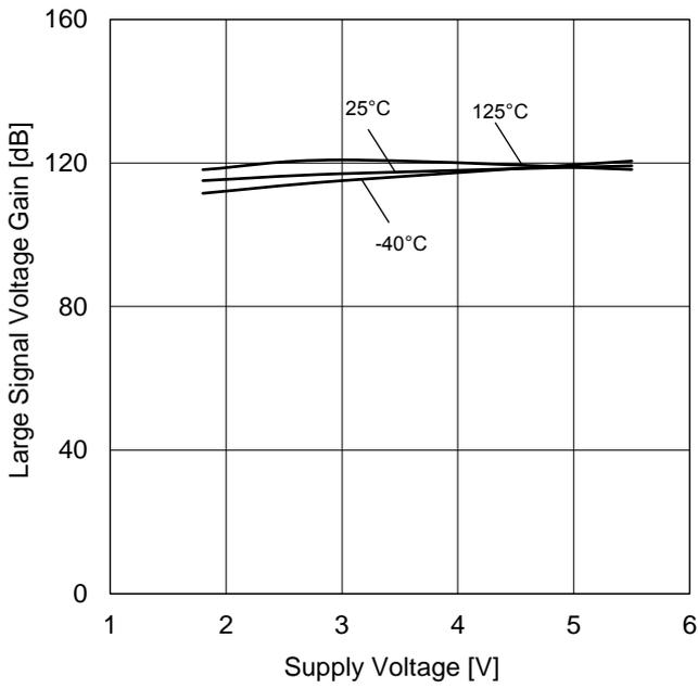
Figure 22. Large Signal Voltage Gain vs Supply Voltage
