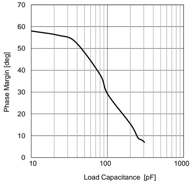
Figure 37. Phase Margin vs Load Capacitance (V<sub>DD</sub>=3.0 V, G<sub>v</sub>=0 dB)
