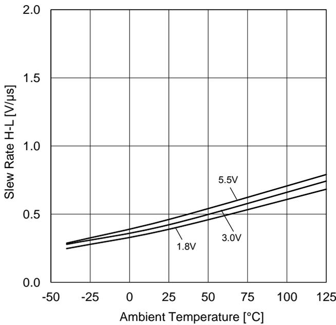
Figure 28. Slew Rate H-L vs Ambient Temperature
