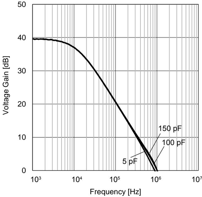
Figure 34. Voltage Gain vs Frequency (V<sub>DD</sub>=3.0 V, G<sub>v</sub>=40 dB)
