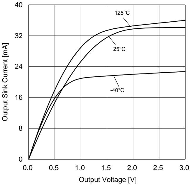
Figure 14. Output Sink Current vs Output Voltage (V<sub>DD</sub>=3.0 V)
