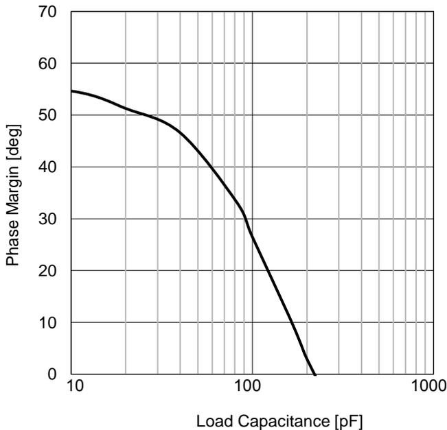
Figure 36. Phase Margin vs Load Capacitance (V<sub>DD</sub>=3.0 V, G<sub>v</sub>=40 dB)
