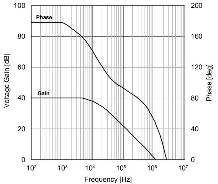
Figure 29. Voltage Gain · Phase vs Frequency (V<sub>DD</sub>=3.0 V)
