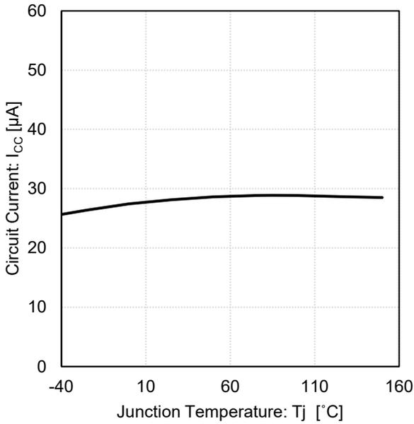
Figure 5. Circuit Current vs Junction Temperature (5 V output)
