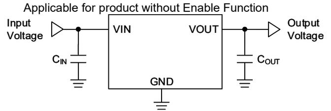
Typical Application Circuits2 (Output voltage adjustable type)
