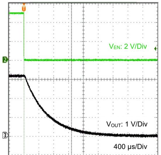
Figure 50. EN Shutdown Waveform
