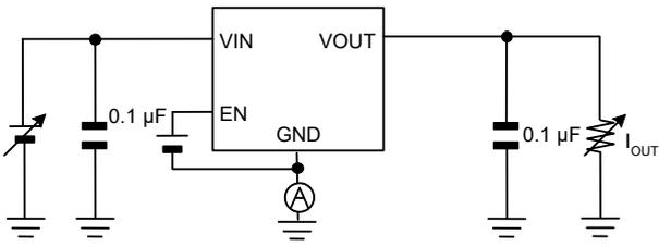
Measurement Setup for Figure 1 to 5, 16, 29 to 33
