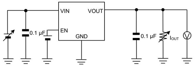
Measurement Setup for Figure 6, 9 to 12, 14, 34, 37 to 39
