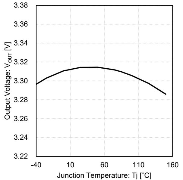
Figure 34. Output Voltage vs Junction Temperature (3.3 V output)
