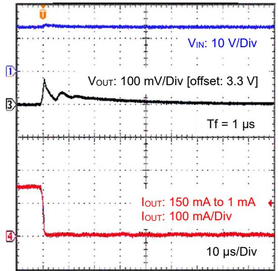
Figure 42. Load Transient 150 mA to 1 mA
