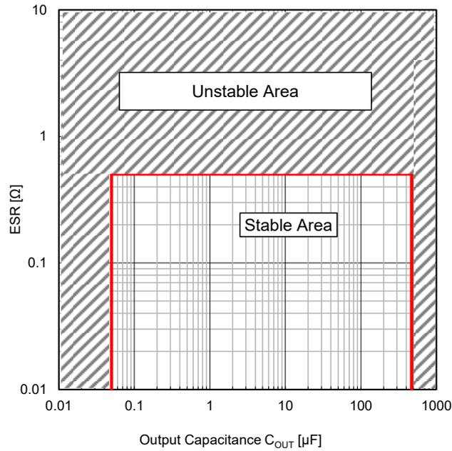
Figure 51. Output Capacitance C<sub>OUT</sub>, ESR Available Area
