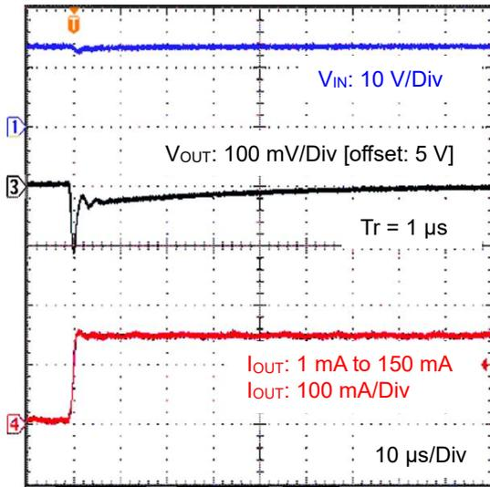
Figure 19. Load Transient 1 mA to 150 mA
