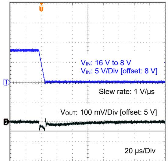
Figure 24. Line Transient 16 V to 8 V
