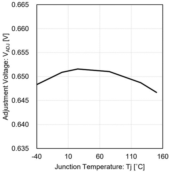
Figure 15. Adjustment Voltage vs Junction Temperature
