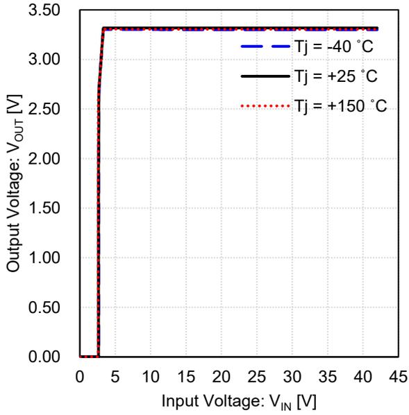
Figure 37. Output Voltage vs Input Voltage (3.3 V output)
