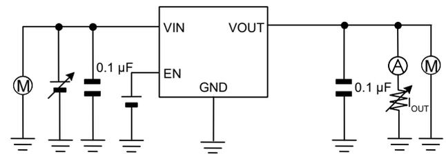
Measurement Setup for Figure 19 to 26, 41 to 48
