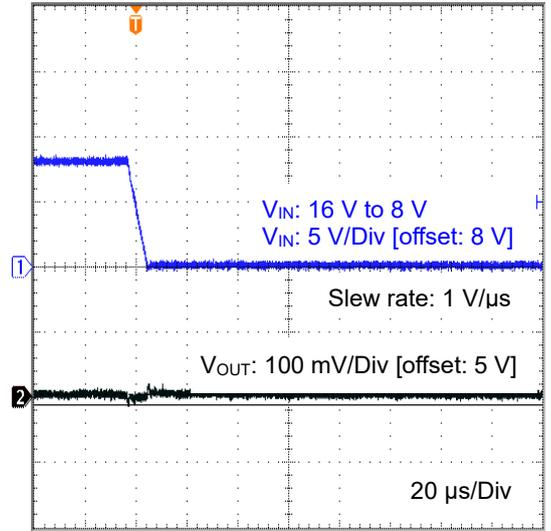
Figure 22. Line Transient 16 V to 8 V
