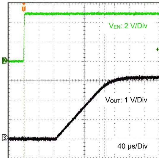
Figure 49. EN Startup Waveform
