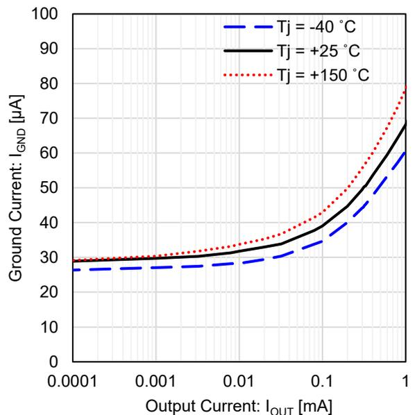
Figure 32. Ground Current vs Output Current
