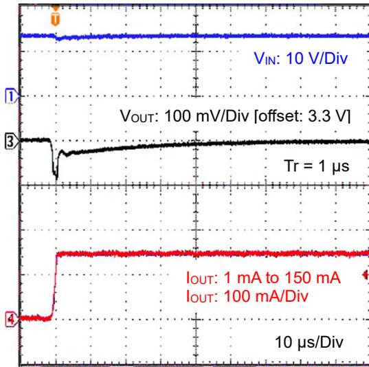
Figure 41. Load Transient 1 mA to 150 mA
