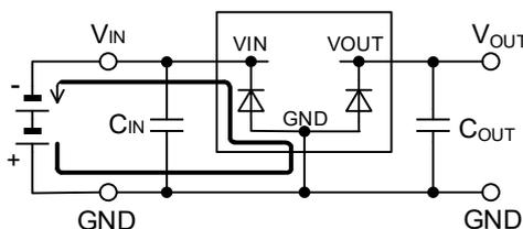
Figure 57. Current Path in Reverse Input Connection
