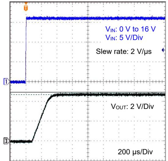
Figure 26. VIN Startup Waveform
