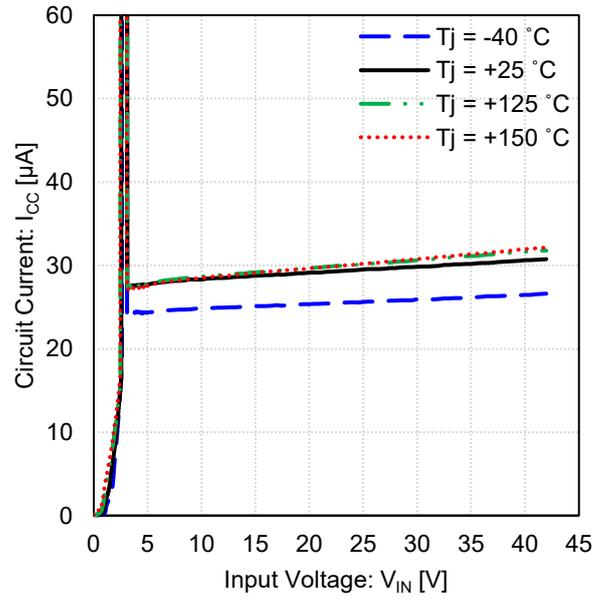
Figure 30. Circuit Current vs Input Voltage
