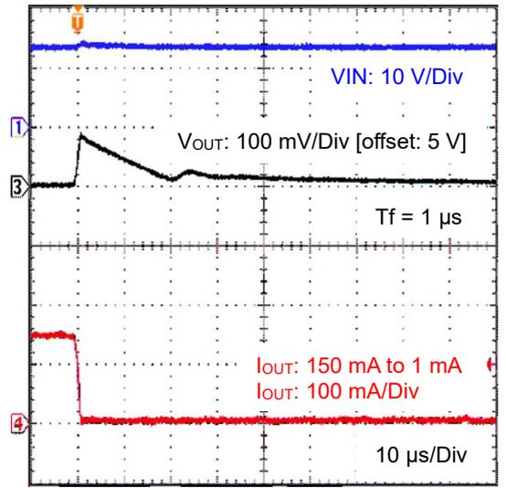
Figure 20. Load Transient 150 mA to 1 mA
