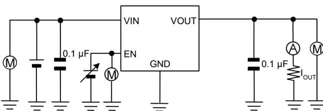
Measurement Setup for Figure 27 to 28, 49 to 50
