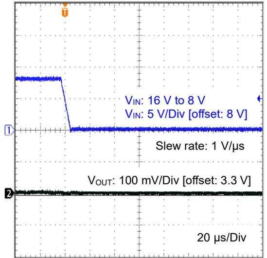
Figure 44. Line Transient 16 V to 8 V
