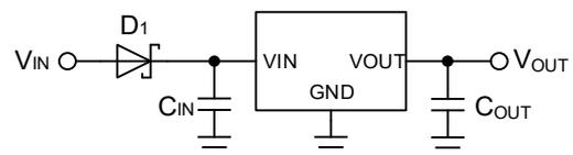
Figure 58. Protection against Reverse Polarity 1
