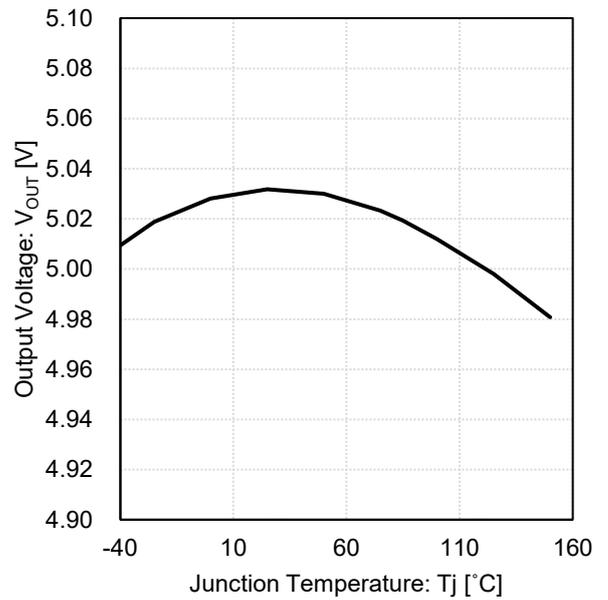
Figure 6. Output Voltage vs Junction Temperature (5 V output)
