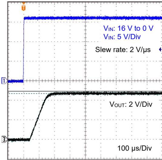
Figure 47. VIN Startup Waveform
