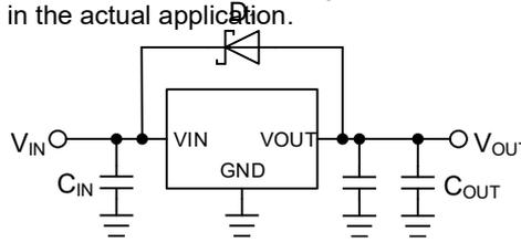
Figure 55. Bypass Diode for Reverse Current Diversion
