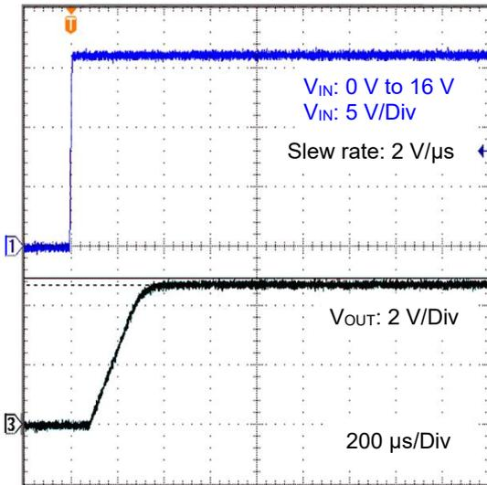
Figure 25. VIN Startup Waveform
