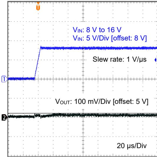
Figure 21. Line Transient 8 V to 16 V
