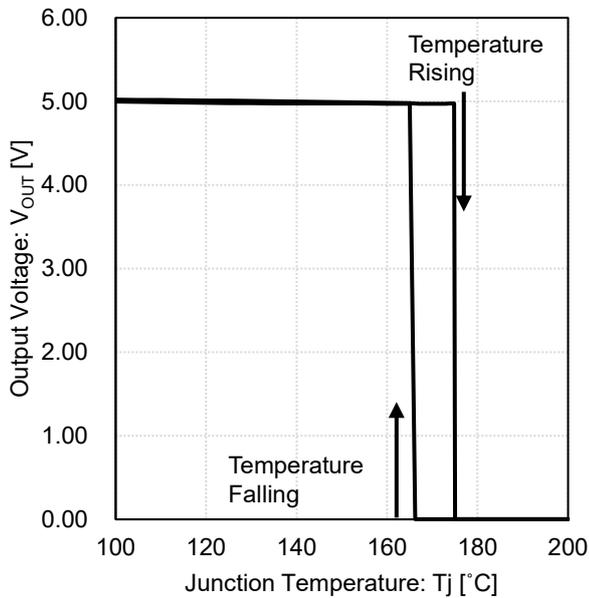
Figure 14. Output Voltage vs Junction Temperature (5 V output)
