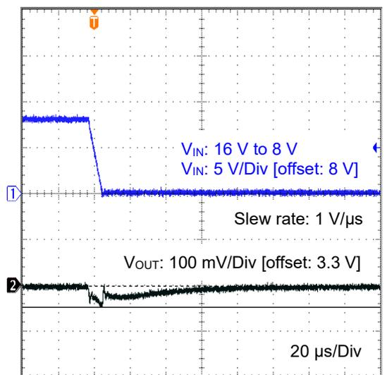
Figure 46. Line Transient 16 V to 8 V
