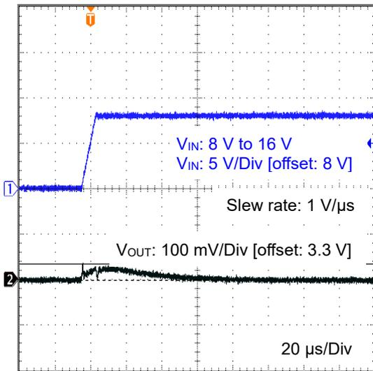
Figure 45. Line Transient 8 V to 16 V
