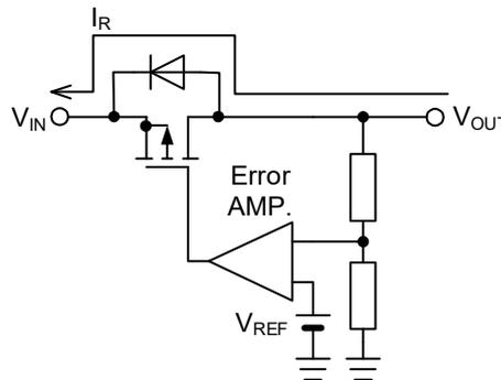
Figure 54. Reverse Current Path in a MOS Linear Regulator
