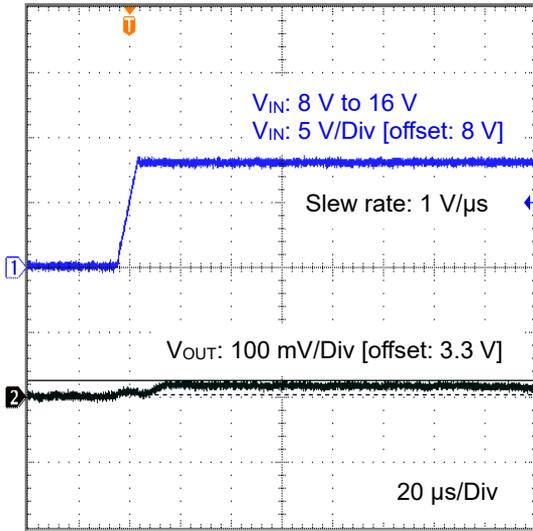
Figure 43. Line Transient 8 V to 16 V
