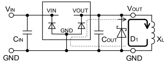
Figure 61. Current Path in Inductive Load (Output: Off)
