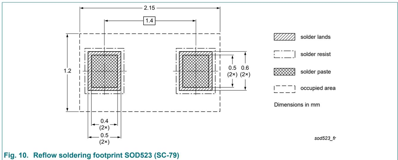
Fig. 10. Reflow soldering footprint SOD523 (SC-79)
